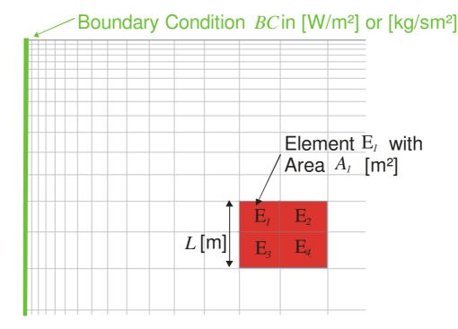
The whole source rate S [W/m] or [kg/ms] which will be evenly distributed over the red marked area is determined as:
