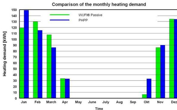
Fig. 4 Comparison of the monthly heating demand for the exemplary building in the ambient climate of Passau, Germany
