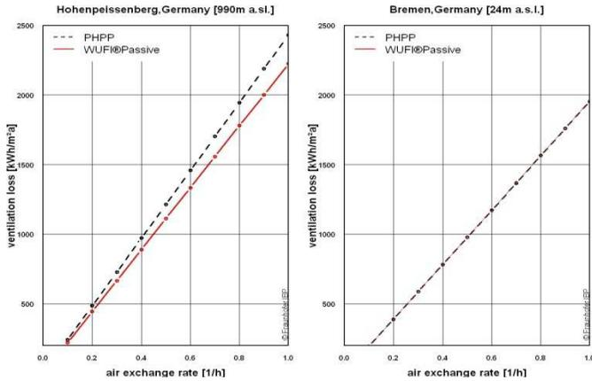
Fig. 2 ventilation heat flows depending on air change rates
