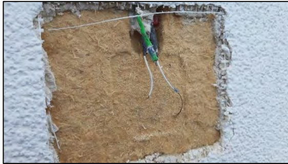
Figure 42 : Opened measuring position P at variant N 2.3 (bright-coloured render) after the test period. No fungal mycelium visible.
