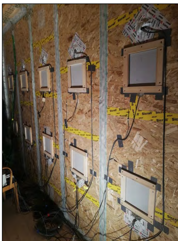
Figure 20 : Measurement setup of a heat flow measurement with heat flow meters and surface temperatures (constellation 1).
