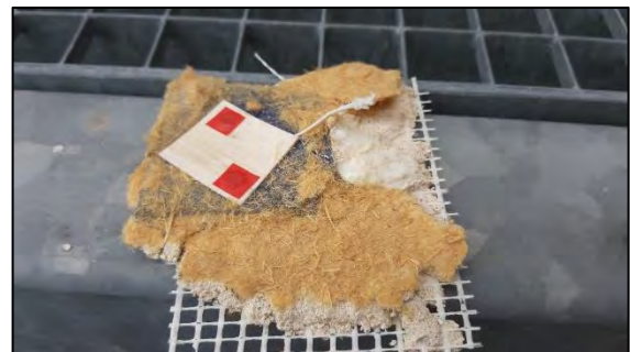
Figure 45 : Removed render layer of variant N 2.6 (dark render) with Balsa sensor and wood fibre residues: No fungal mycelium visible.
