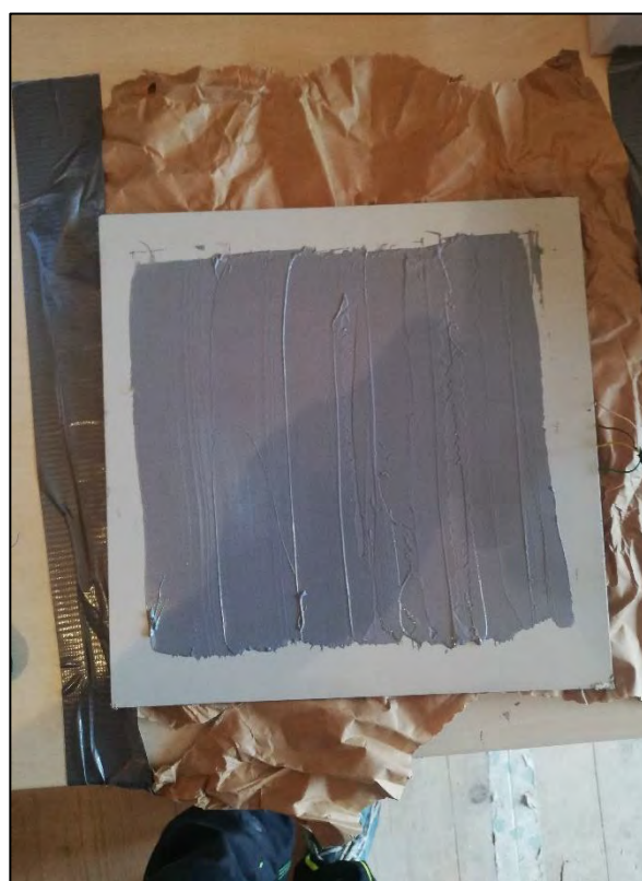
Figure 21 : Heat flow meter with applied thermal paste ( \lambda = 6 \text{ W/mK} ).
