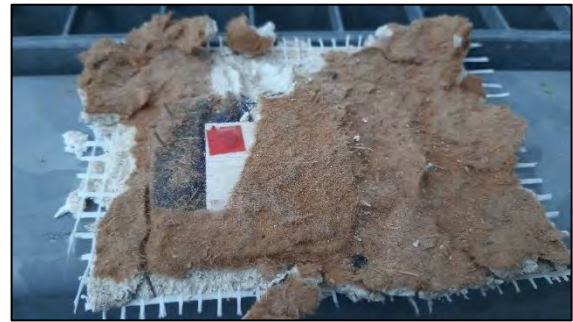
Figure 50 : Removed render layer of variant N 2.8 (bright-coloured render) with Balsa sensor and wood fibre residues. No fungal mycelium visible.
