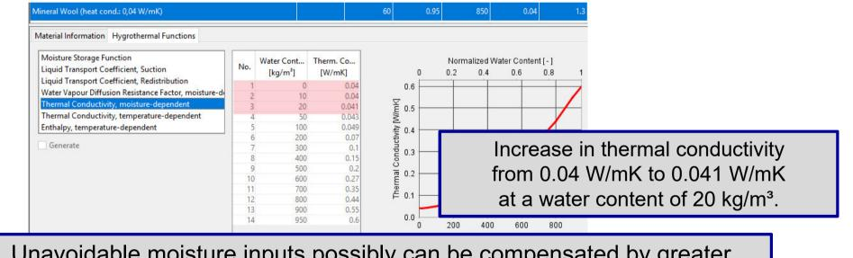
Unavoidable moisture inputs possibly can be compensated by greater insulation thicknesses if the moisture has no other negative effects.
