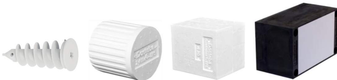
Fig. 22 Examples of fastening loads in internally insulated structures: on the left spiral anchors for light loads (source: www.ejot.de ), in the middle two compression-resistant mounting elements for medium loads (source: www.dosteba.de ), on the right heavy-duty anchors with thermal decoupling for heavier loads (source: www.dosteba.de ).
