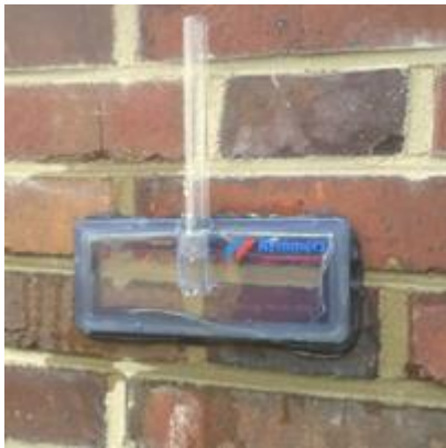
Fig. 25 Testing plate according to Franke, detection of water content in brick and joint
