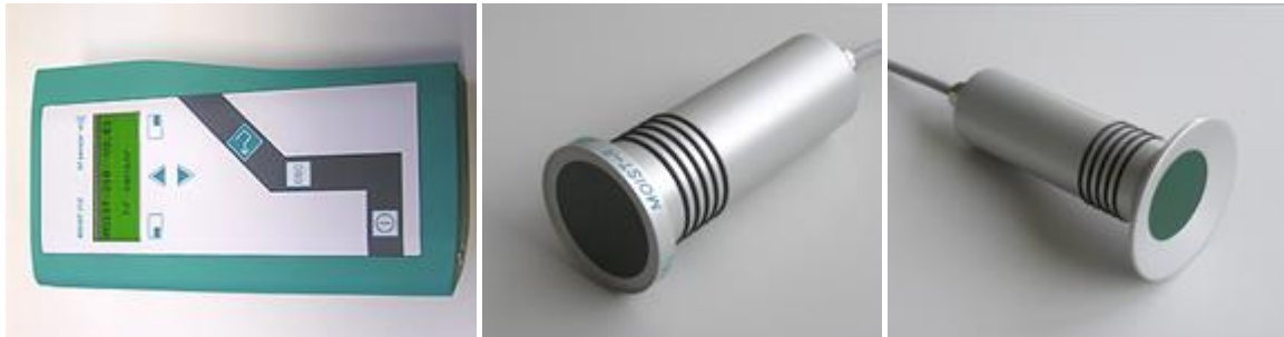
Fig. 21 Microwave moisture meter with different measuring heads (hf-sensor.de)
