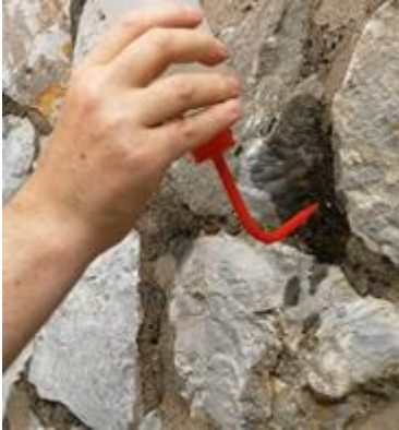
Fig. 23 Wetting test on a natural stone façade
