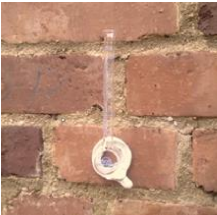
Fig. 24 Test tubes according to Dr. Karsten, placed on a brick
