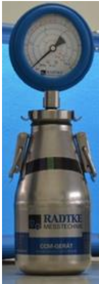
Fig. 22 CM measuring device for humidity measurement (radtke-messtechnik.com)
