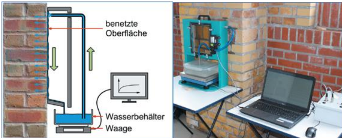
Fig. 26 Water absorption measuring device, measuring principle and practical application [hf-sensor.de]
