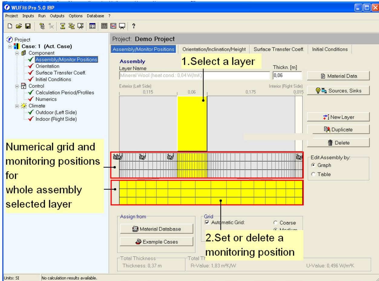
Select the layer where you like to insert a monitoring position. The numerical grid of the selected layer is then shown zoomed in the lower grid bar. Insert or remove a monitoring position by clicking on the desired element of the grid. Monitoring positions can only be set in the centre of a grid element and not between two elements.
