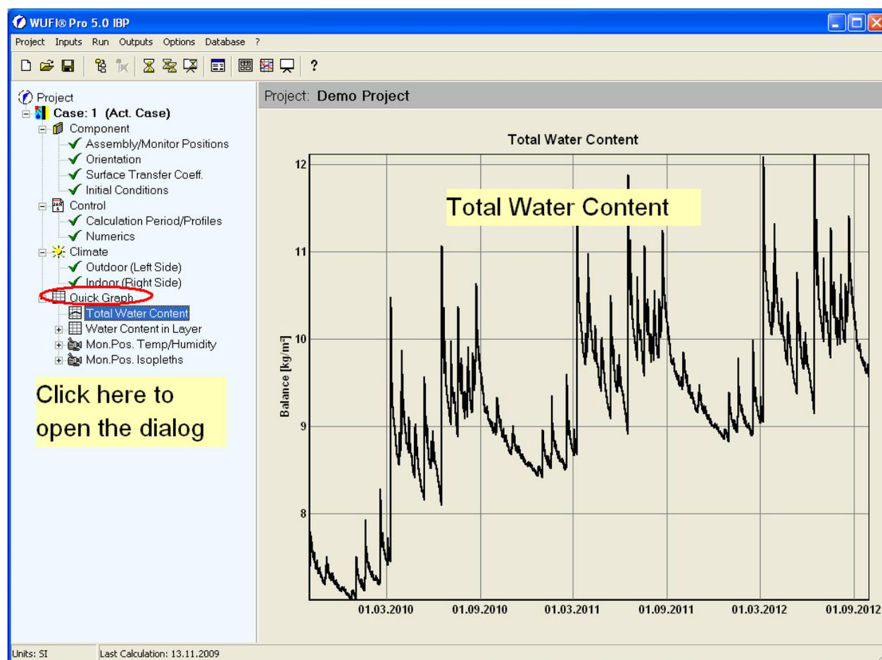
Usually, the main criterion for assessing the results is the behaviour of the total water content. It shows whether moisture has accumulated or dried out during the investigated period.
