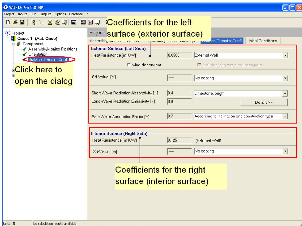
In the example case, „outer wall“ conditions are assumed for the heat transfer. For the radiation absorptivity we select a light lime stone. As appropriate for a vertical wall a rain absorption of 70% is selected.
