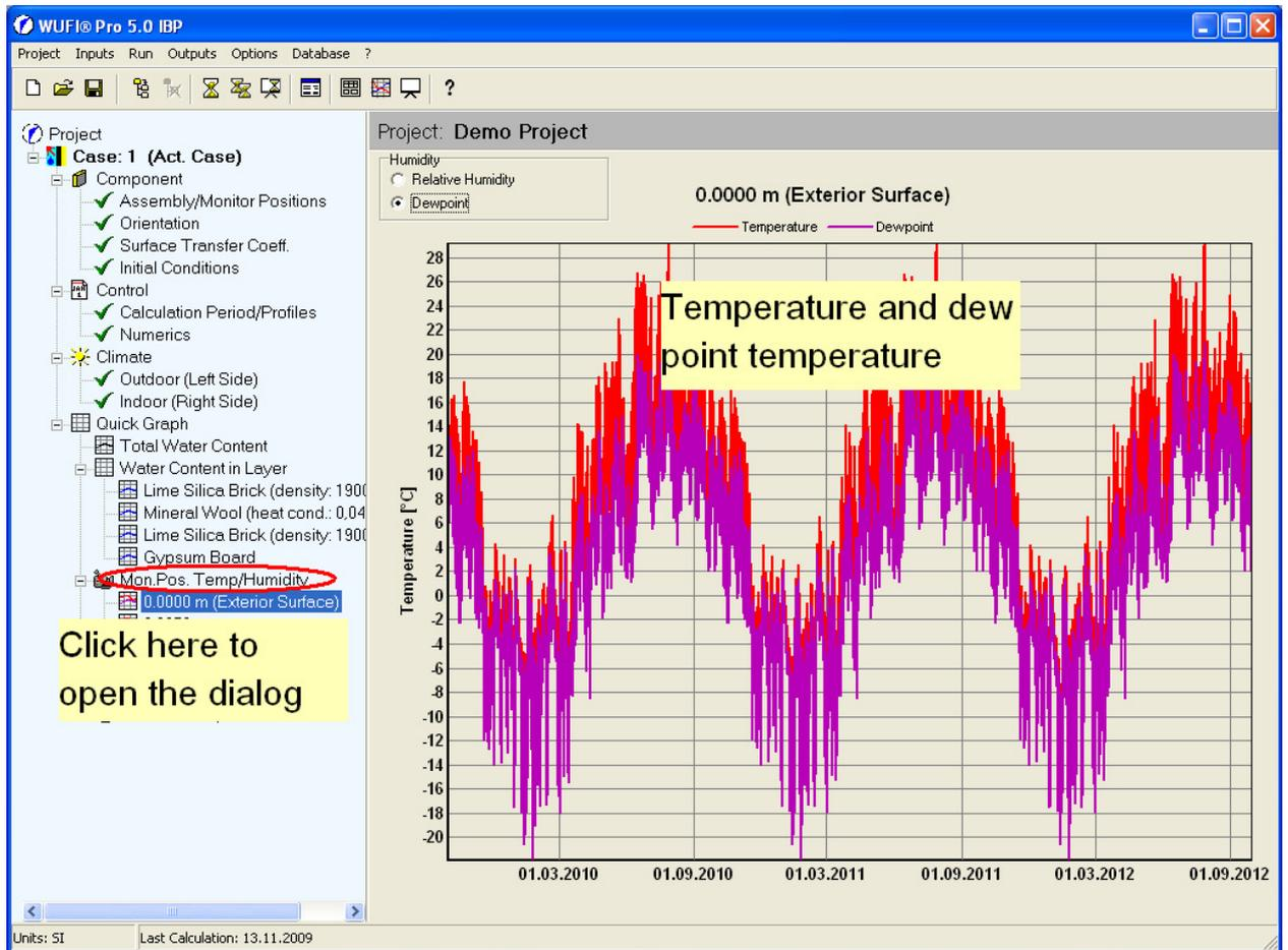
The diagram displaying the temperature and the dew point at the monitoring positions allows you to examine whether the temperature falls below the dew point at any time during the investigated period. This is the case when the red curve (temperature) is lower than the purple curve (dew point).
