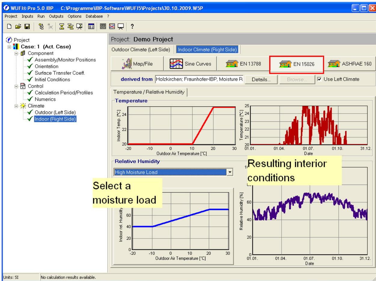
Specifically, the indoor temperature is kept at 20 °C for outdoor temperatures below 10°. For outdoor temperatures between 10 °C and 20 °C the indoor temperature varies in linear dependence of the outdoor temperature. For outdoor temperatures above 20 °C the indoor temperature is kept constant at 25 °C.
