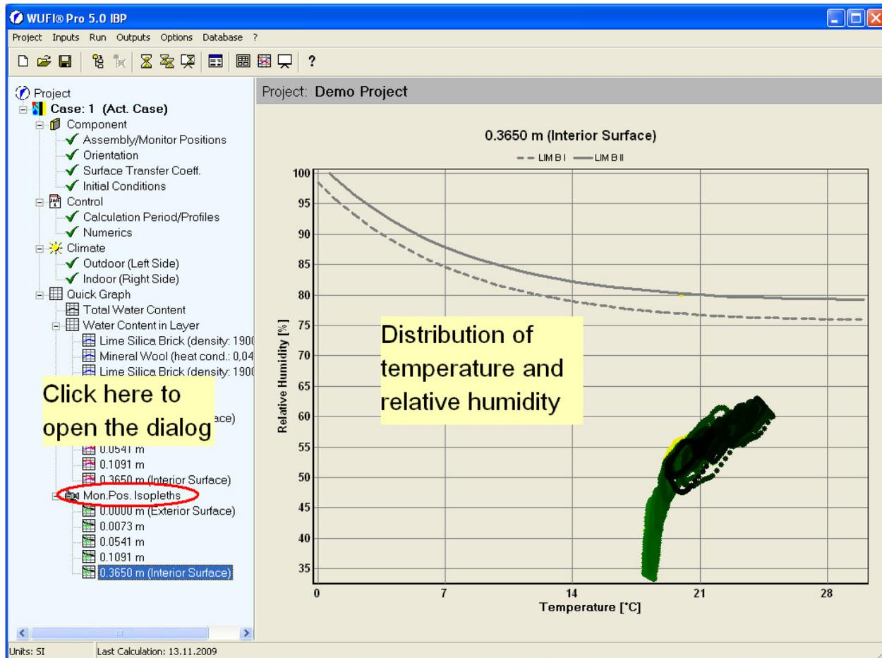
For each monitoring position, the quick graph „Mon.Pos Isopleths" plots the relative humidities at each time step against the simultaneous temperatures. This enables you to assess whether conditions of high temperature and high humidity occur at the same time which may create problems for some materials.
