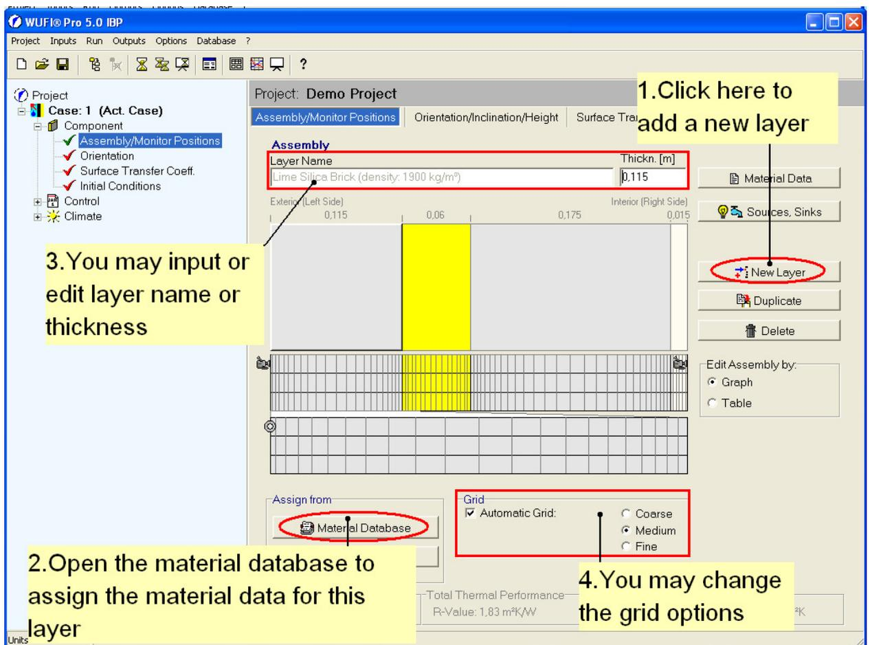
Use the button „New Layer“ to create a new layer on the right side of the component. If needed, use the mouse to drag the layer to the desired location in the assembly. Then assign the appropriate material to the new layer using the button “Material Database” again.
