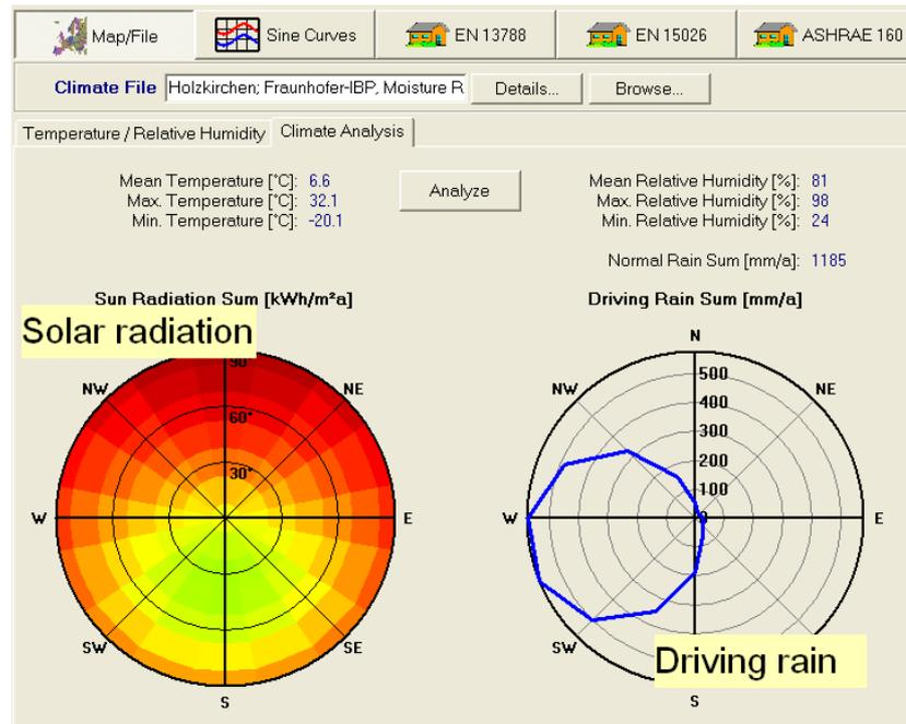
The rain rose shows the yearly driving rain sum on vertical surfaces for different orientations. The scale of this diagram is adapted to accommodate the maximum driving rain load occurring at this location. The amount of driving rain is given in mm/year.
