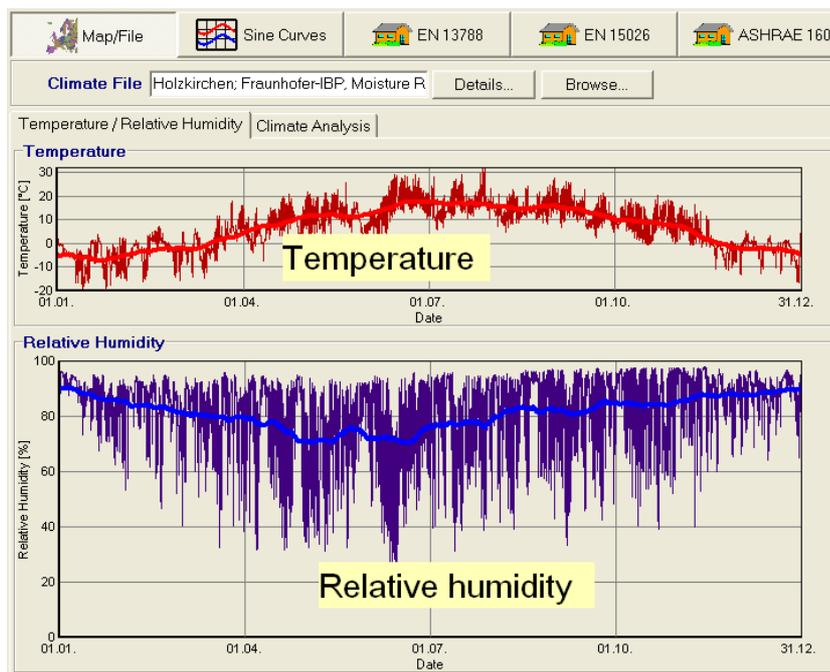
The climate module can also perform a more detailed analysis of the climate file, providing the minimum, maximum and mean values of temperature and relative humidity, the yearly amount of normal rain and the directional distributions of solar radiation and driving rain.
