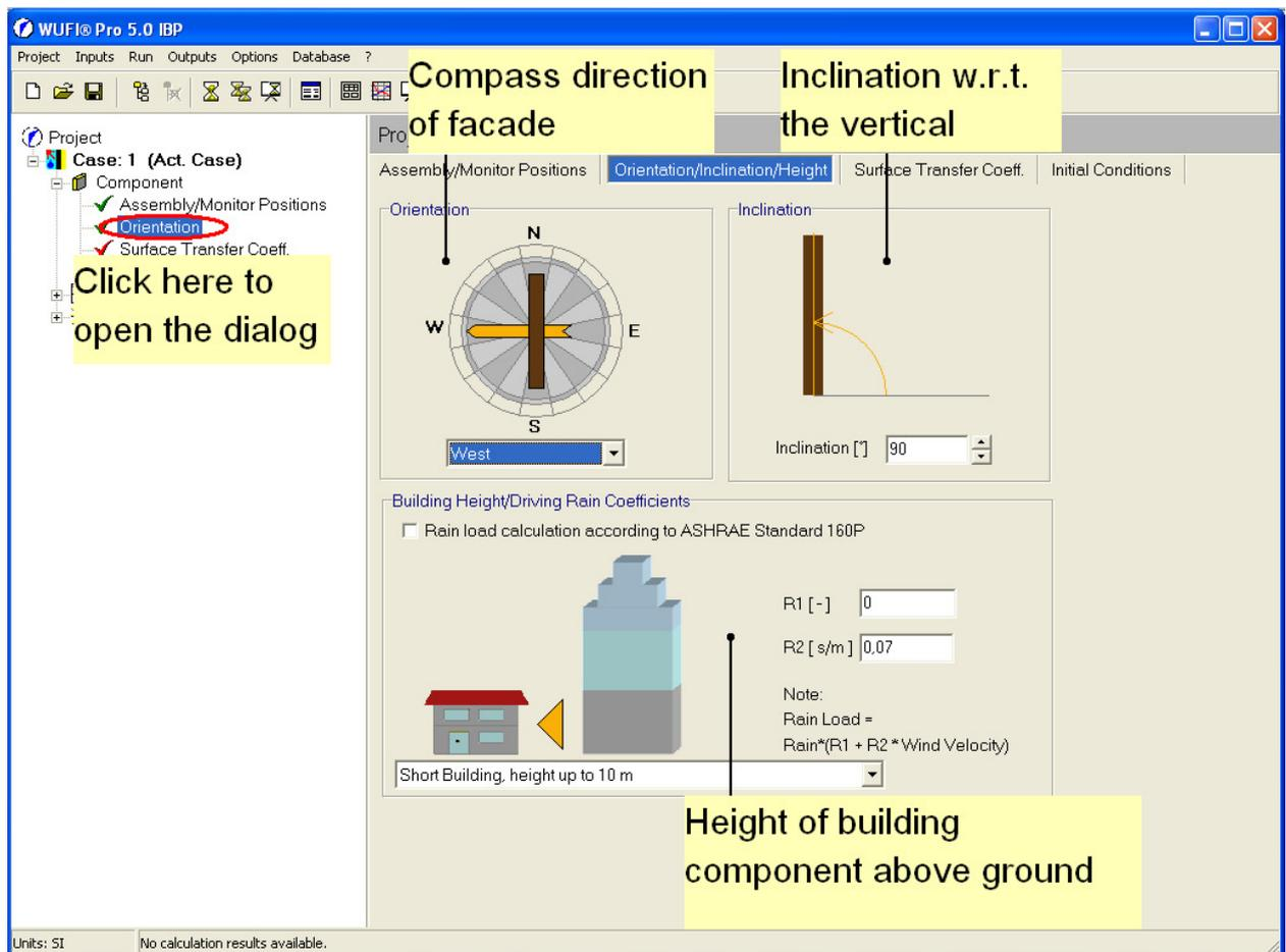
In the example case the choices are: orientation: west; inclination: 90°; height: "Short Building, height up to 33 ft".
