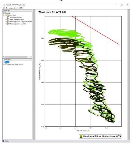
The relative pore air moisture in the interior centimetre of the sheathing doesn't exceed the limits according to WTA.
