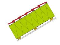
For this purpose, the wood moisture content is evaluated in [% by mass] in the outer centimeter of the wood-fiber insulation in the settled state. The settled stage has reached if the course of the water content does not change inbetween the years any longer.
