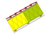
For the evaluation of the wooden sheathing, the course of the wood moisture content in [% by mass] in the wooden sheathing in the settled state is used. The value of 20 % by mass for wood and 18 % by mass for wood-based materials specified in DIN 68800 [2] is recommended as the limit value. If this limits are kept, no further evaluation is necessary.
