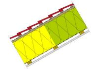
However, this limit value includes high safety margins and, in contrast to the WTA guideline 6-8 [9], no specifications are made for the evaluation area. In the case of thin wooden sheathings, the entire section of the sheathing shall be evaluated, otherwise the most critical 1 cm thick section should be used in accordance with the WTA evaluation.
