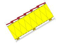
The amount of condensation occurring below the roofing felt is used for result evaluation. For this purpose, the maximum water content in [kg/m³] in the outer area of the mineral wool insulation is evaluated. A distinction is made here between insulation materials with an internal moisture storage function and those with a measured moisture storage function. For more detailed information, please refer to the <u>Guideline for assessing condensation problems in hydrophobic material fiber</u>.
