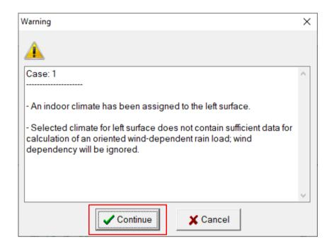
This warning appears at the start of the calculation and can be ignored for the calculation of an interior component
