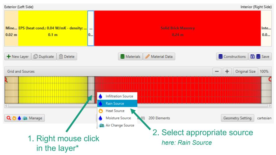
\*) Driving Rain source is inserted in the outer 5 mm of the layer behind the insulation.
