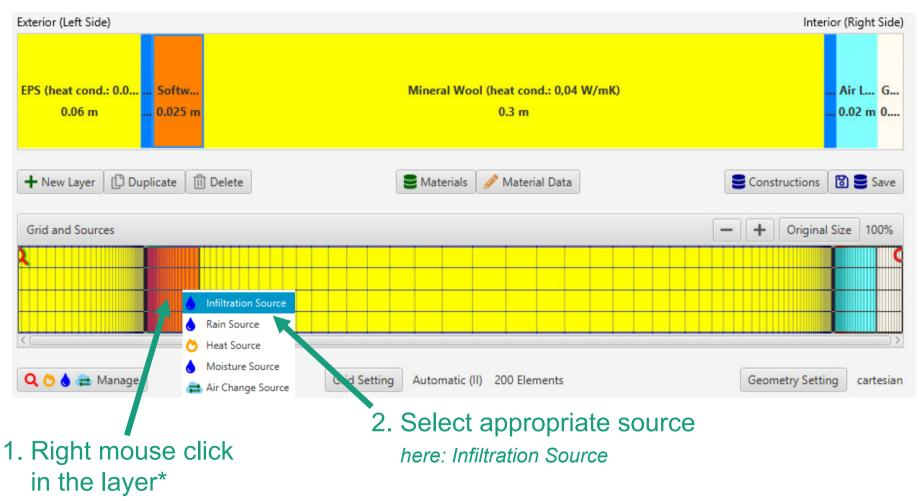
\*) Material in which condensation is to be expected due to convection. Infiltration source either in the inner 5 mm of the wooden sheathing or – if there is no sheathing – in the outer 5 mm of the insulation between the rafters.
