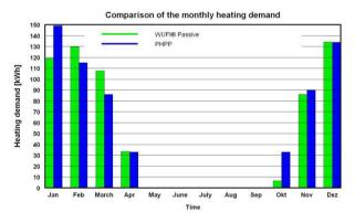
Fig. 4 Comparison of the monthly heating demand for the exemplary building in the ambient climate of Passau, Germany
