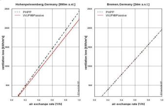
Fig. 2 ventilation heat flows depending on air change rates
