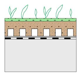
sedum planting substrate type L incl. drainage board FKD 25 protection mat
