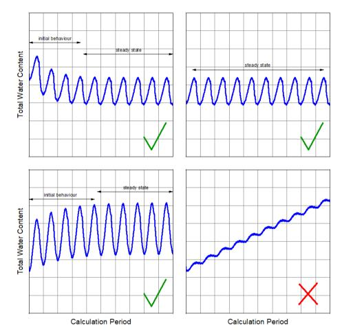
Evaluation of the moisture balance is only the first step, the analysis must always include the water contents in the layers!!!
