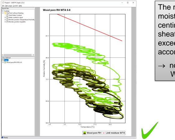
The relative pore air moisture in the interior centimetre of the sheathing doesn't exceed the limits according to WTA.
