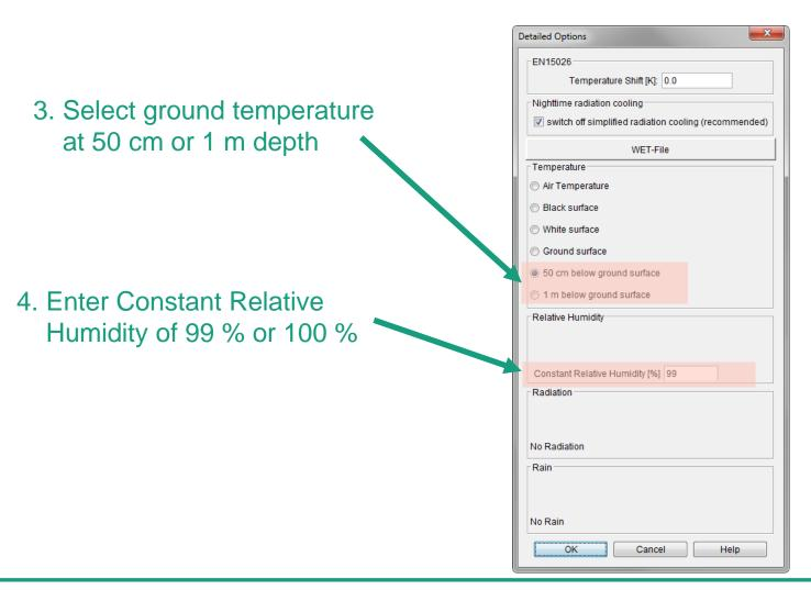
Soil temperature setup (from diagram)
