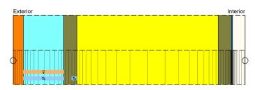
As the occurring air exchange rates are often not known, it may be useful to vary the air exchange rate to see its influence on the hygrothermal behavior of the construction. (Air exchange rates are usually between 10 and 200 1/h)
