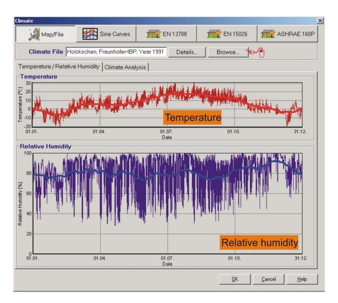
WUFI 2D also offers analyses of average and extreme values for temperature and relative humidity and the distributions of solar radiation and driving rain. Access these by clicking on the tab "Climate Analysis".
