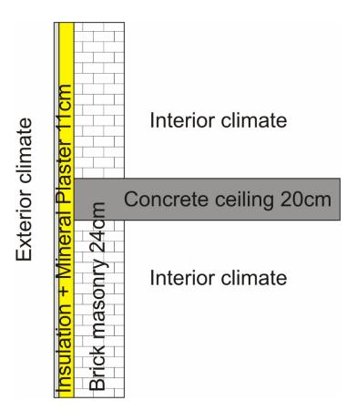
The building component consists of a 20 cm thick concrete ceiling supported by a 24 cm thick honeycomb brick wall. An exterior insulation and finish system (EIFS) composed of mineral wool insulation (10 cm thick) and mineral plaster (1 cm thick) has been applied to the outside of the wall.
