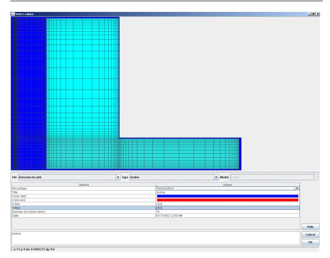
Right-click on the grid and from the pop-up menu choose "Select total construction". From the drop-down list "Result type" choose "Temperature". Then select the desired point in time as the "Date" and click "OK". WUFIGraph displays the temperature distribution in the component at this point in time as isolines.
