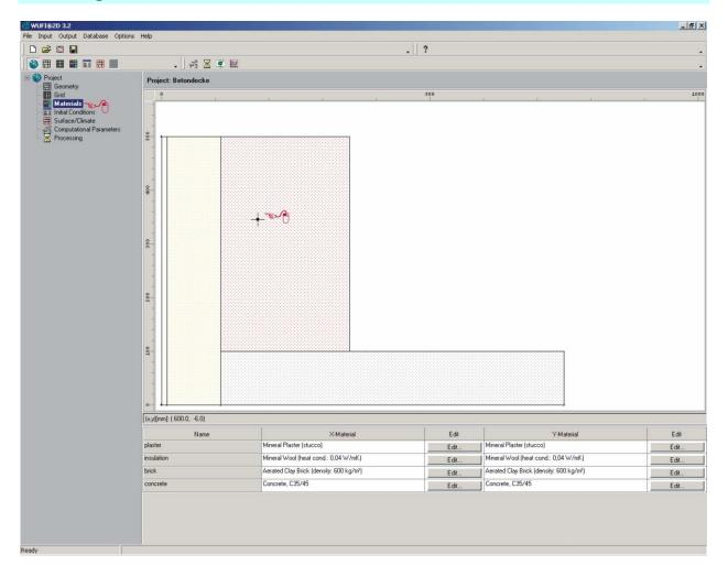
Click on the explorer tree item "Materials" to open the dialog panel shown above. It shows the building component as defined previously. Click on one of the retangles to assign the material properties.
