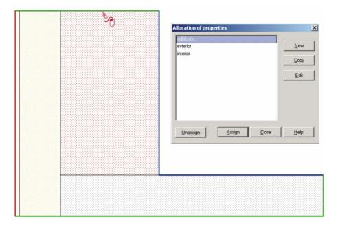
The screenshot above shows the building component and the dialog "Allocation of properties" with the three sets of boundary conditions used in the example (the "adiabatic" set of boundary conditions has been assigned to the three surface segments marked green in the diagram, the "exterior" conditions to the red segment and the "interior" conditions to the two blue segments).
