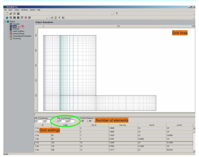
Click on the explorer tree item "Grid" to open the dialog panel shown above. WUFI 2D displays the construction you defined in the previous step and overlays it with an automatically generated numerical grid. You may use this dialog to finetune the grid if needed.
