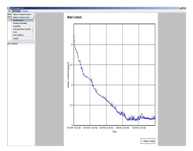
The behavior of the total water content allows a first assessment of the results. It shows whether the overall water content of the component increases or decreases during the period under investigation.
