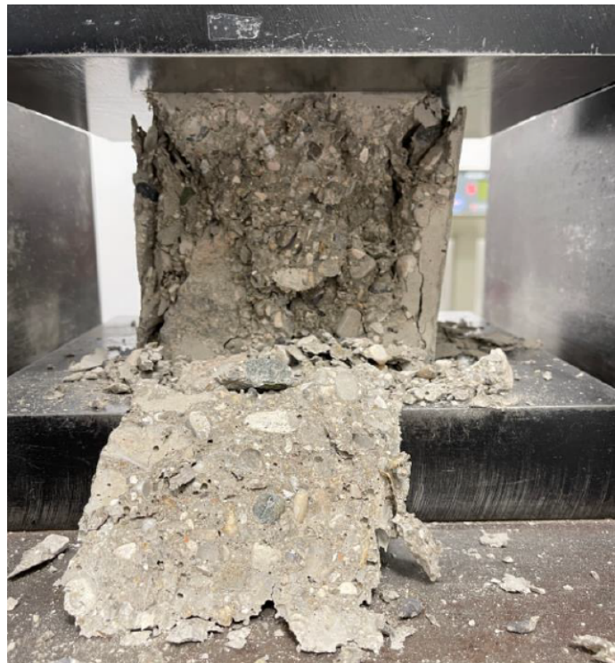
Figure 29: Cube specimen type C-3 after compressive strength testing
