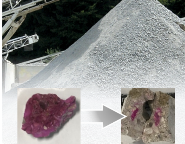
Figure 44: Processing and storage of concrete recyclate in landfills (background), typical degree of carbonation of the aggregates (bottom left), advanced carbonation (bottom right)
