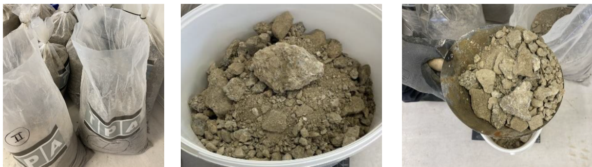
Figure 17: Example of the samples received (illustrated RB II 0/63, U7, U-A) of the processed recycled aggregates
