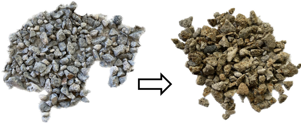
Figure 14: Coarse recycled aggregates before and after the acid attack
