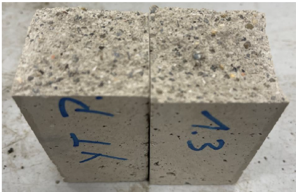
Figure 30: Fracture surface of prism specimen type P-1 after bending tensile testing
