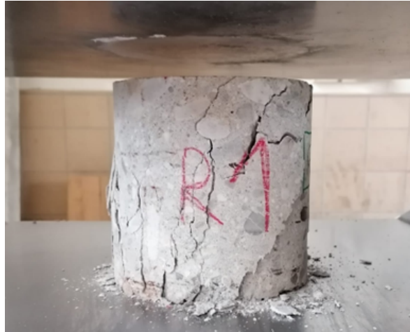
Figure 27: Compressive strength testing of cylindrical specimen
