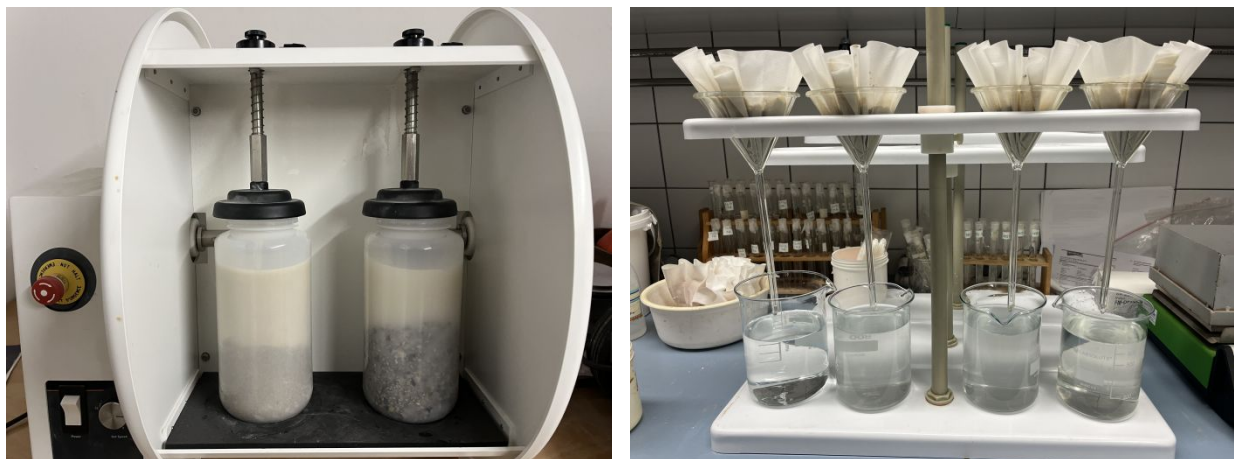
Figure 5: RCA in overhead shaker for 24 h (l), filtered Eluate (r)
