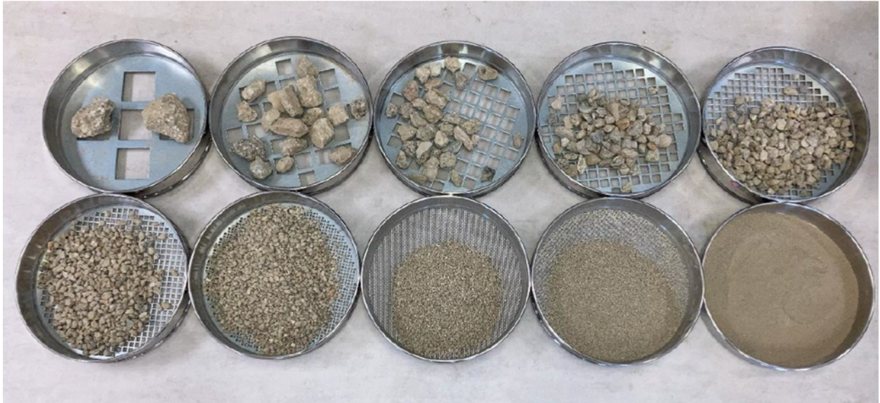
Figure 21: Evaluation of the residue in the analysis sieves of concrete recylate RB II 0/63, U7, U-A
