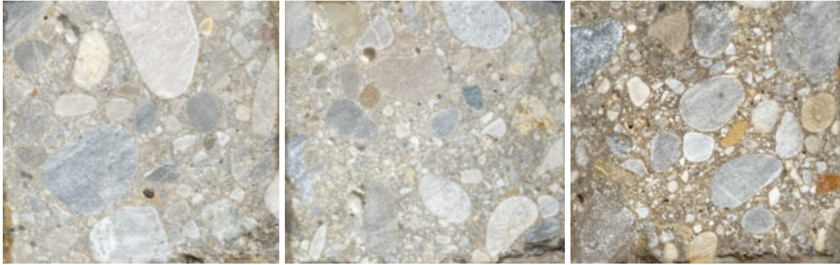
Figure 70: The varying ratio between cement matrix and aggregates of the exemplary specimens influences the material properties and thus leads to a certain variation of their parameters.
