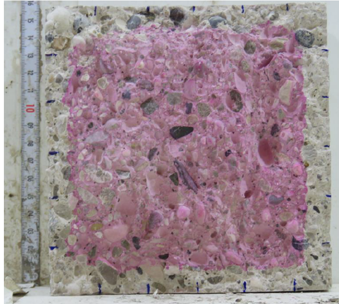
Figure 117: Split cube specimen of standard mix design C-0
