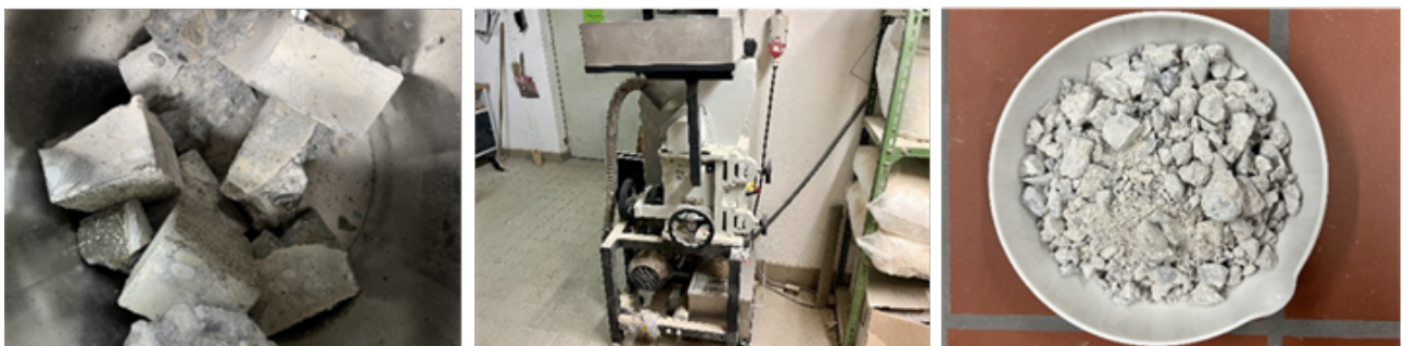
Figure 3: Demolition material (l), jaw crusher (m), RCA material with a grain size of 0–16 mm (r)
