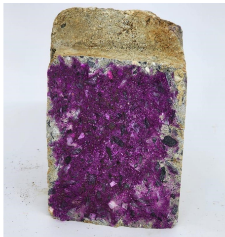
Figure 13: Paver's surface showing that carbonation is restricted to its borders
