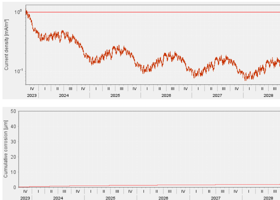
Figure 104: WUFI Corr results – ETICS with mineral fibre insulation: top: Corrosion current flow at reinforcement level. bottom: Total corrosion loss over a period of 5 years.
