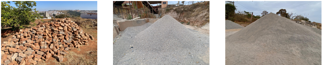
Figure 12: Materials used for research. Left: Concrete pavers; center: coarse recycled aggregate; right: fine recycled aggregate.
