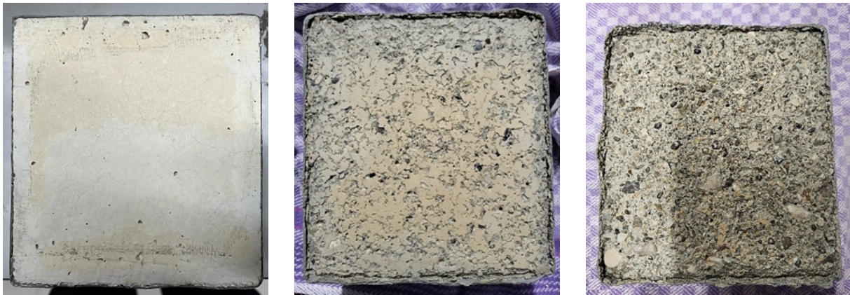
Figure 11: Visual changes in the surface of the CIF test specimens CI-L after 0 cycles (l), 28 cycles (m) and 56 freeze-thaw cycles (r)
