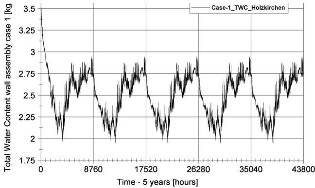
**Figure 4** Total water content (WC) wall assembly—Case 1: Holzkirchen, north orientation.
