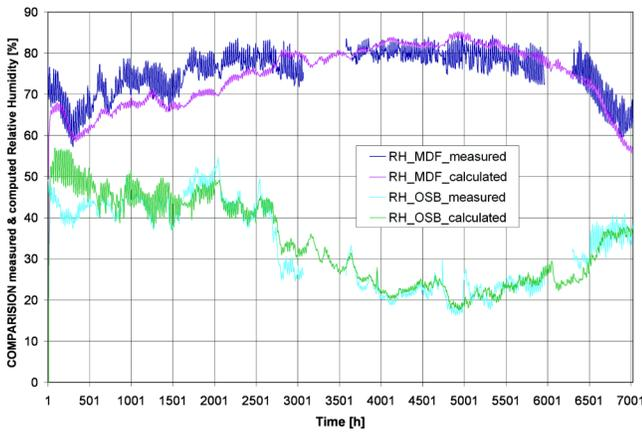
**Figure 22** Comparison of measured and computed relative humidity of the surfaces of OSB and MDF boards—Case 1: Measured climate, south Austria.
