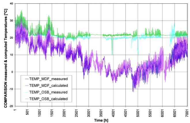
**Figure 23** Comparison of measured and computed temperatures on the surfaces of OSB and MDF boards—Case 1: Measured climate, south Austria.
