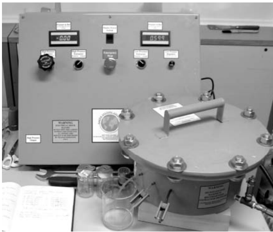
FIG. 1: Pressure plate apparatus, compressor and high pressure chamber. FIG. 2: Test specimens on fine meshed cloth, kaolin clay and ceramic plate in the chamber.
