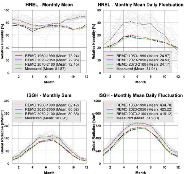
Figure 7 Comparison of REMO 1960-1990, 2020-2050 and 2070-2100 climate data and measured long time weather data for Roggersdorf
