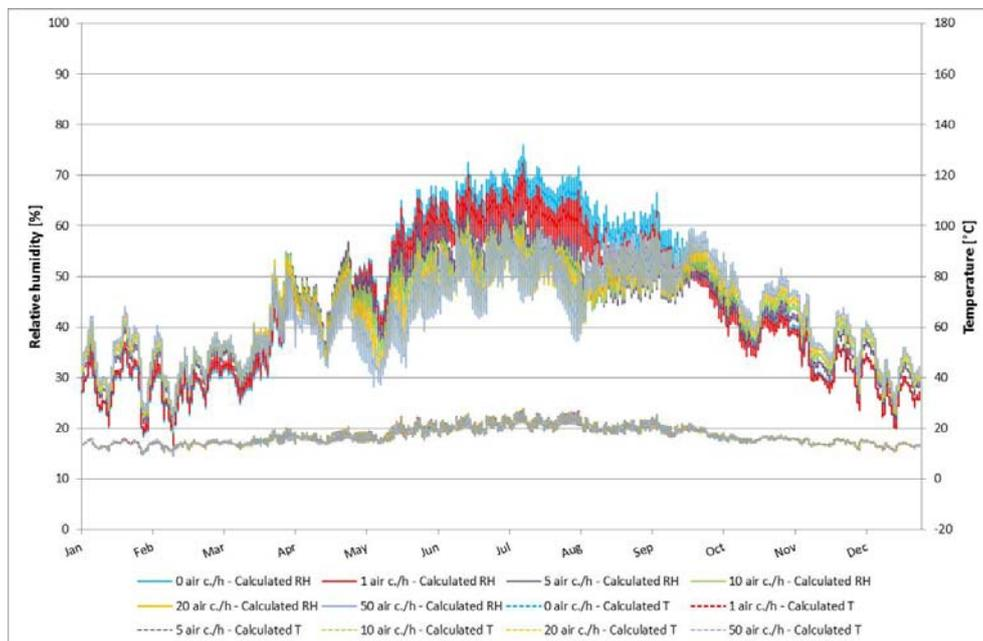
Chart 3: Position C. Calculated relative humidity and temperature with different applied air flow in the air gap. Different colors show different flow.
