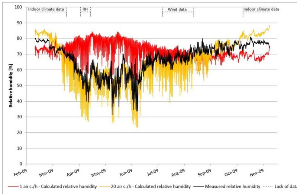
Chart 6: Example on comparison in position B. Measured relative humidity (black). Calculated relative humidity for 1 air changes per hour (red). Calculated relative humidity for 20 air changes per hour (yellow). Periods with gaps in boundary conditions are shown in the top.
