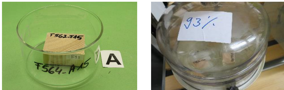
fig. 4 : Glass dish with sample (left) and desiccator with samples (right) (Source: IBP)
