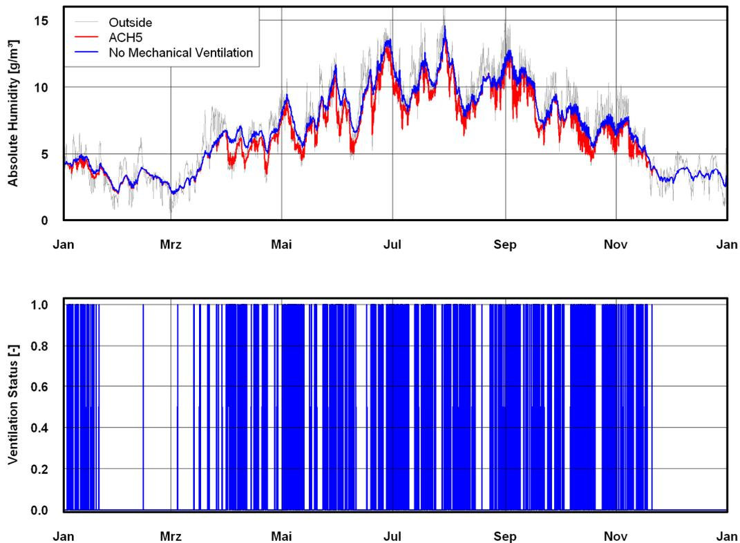
**Figure 4.** Absolute humidity outside and inside the church as well as ventilation status during the whole simulation period
