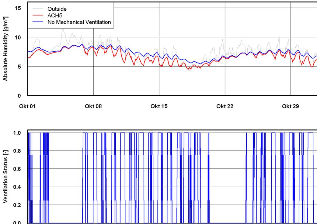
**Figure 5.** Absolute humidity outside and inside the church and ventilation status for simulation in October
