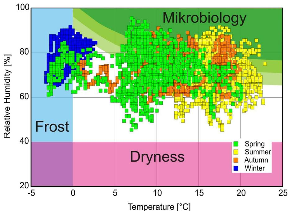
**Figure 1.** Temperature and humidity during 2005. Half of the time rh lies above 75 %, during winter the church freezes for 6 weeks.
