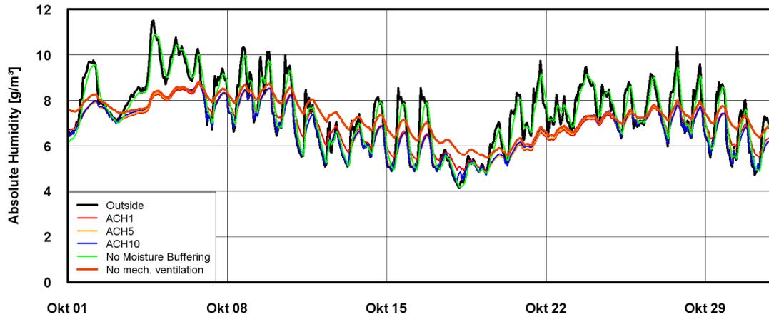
**Figure 6.** Absolute humidity outside and inside the church with different parameters for simulation during representative month October
