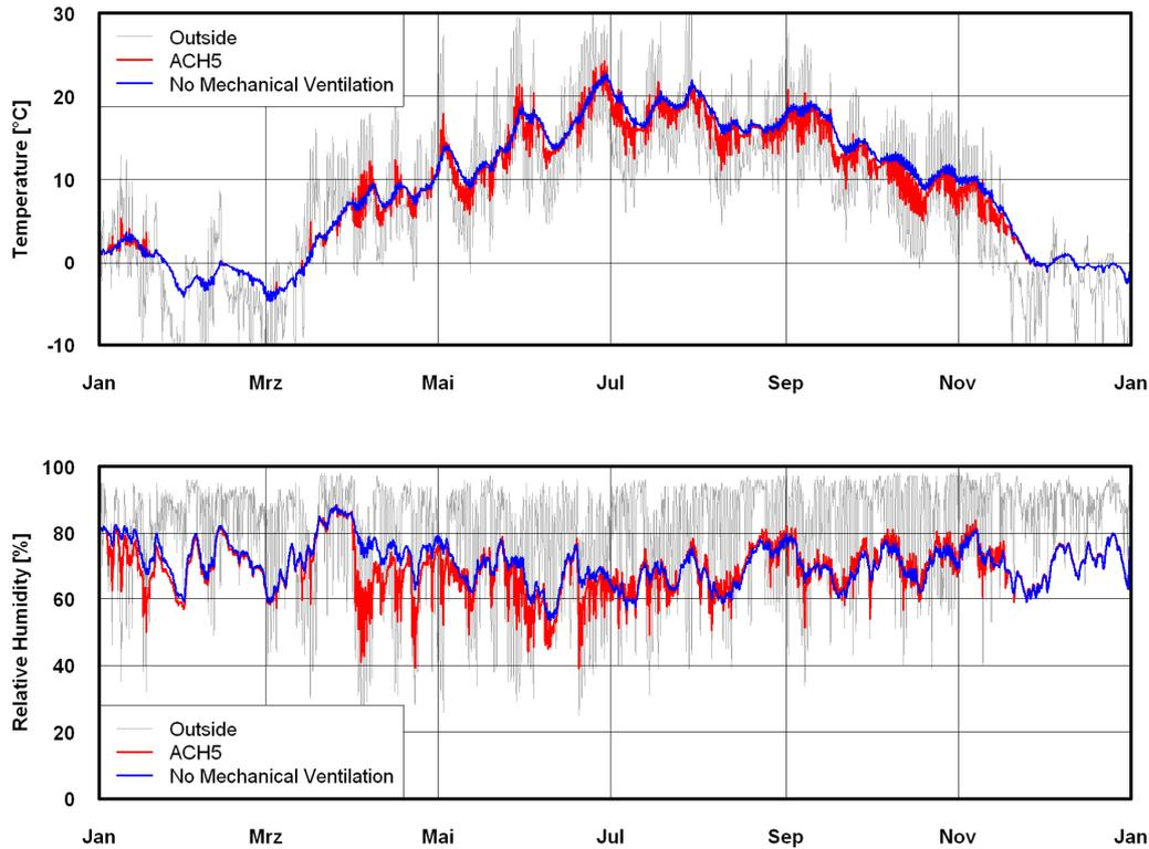
**Figure 3.** Temperature and relative humidity outside and modelled conditions inside the church during the whole simulation period with (Air Exchange 5 1/h) and without mechanical ventilation
