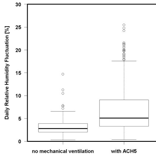
**Figure 8.** Boxplots of simulation results for all daily fluctuations of relative humidity in the space without ventilation and the space with ACH 1/h
