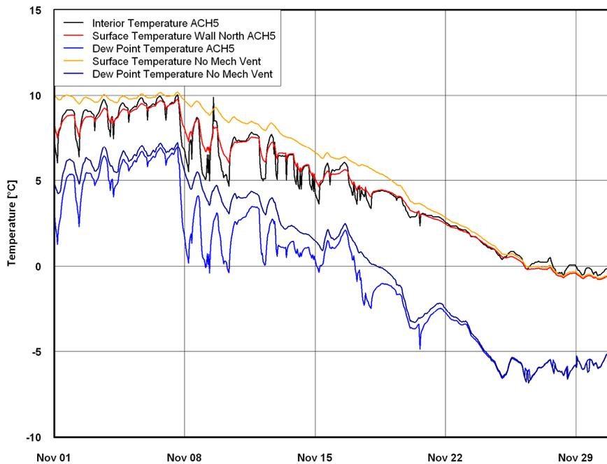
**Figure 7.** Surface temperature and dew-point temperature for North wall without mechanical ventilation and with ventilation control and ACH 5 1/h
