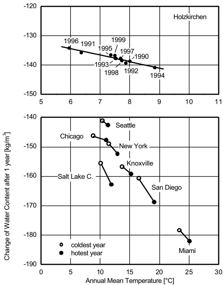
Figure 7: Change of water content in the AAC flat roof after one year under different climates in Germany and United States.
