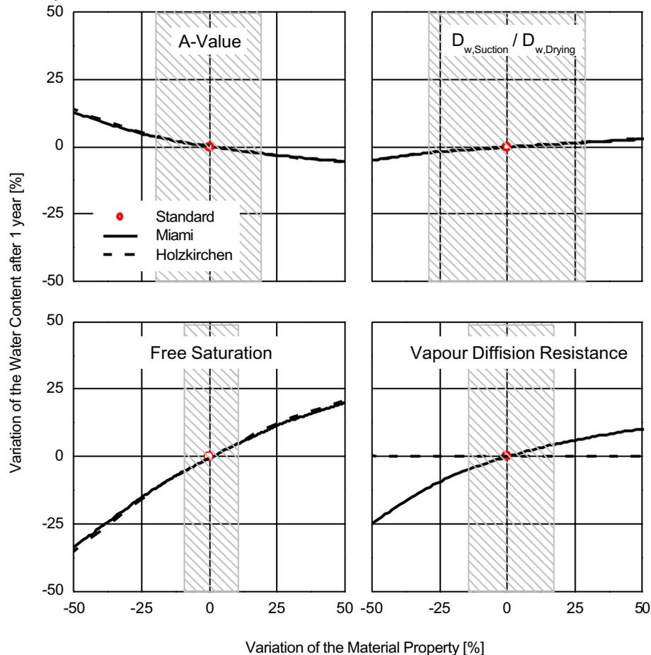
**Figure 5: Sensitivity Analysis for the transient drying behaviour of the AAC flat roof under typical climate conditions for Holzkirchen for the first year.**
