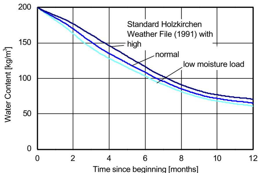
**Figure 6: Drying behaviour of the AAC flat roof during the first year under typical climate conditions for Holzkirchen and different interior moisture loads.**
