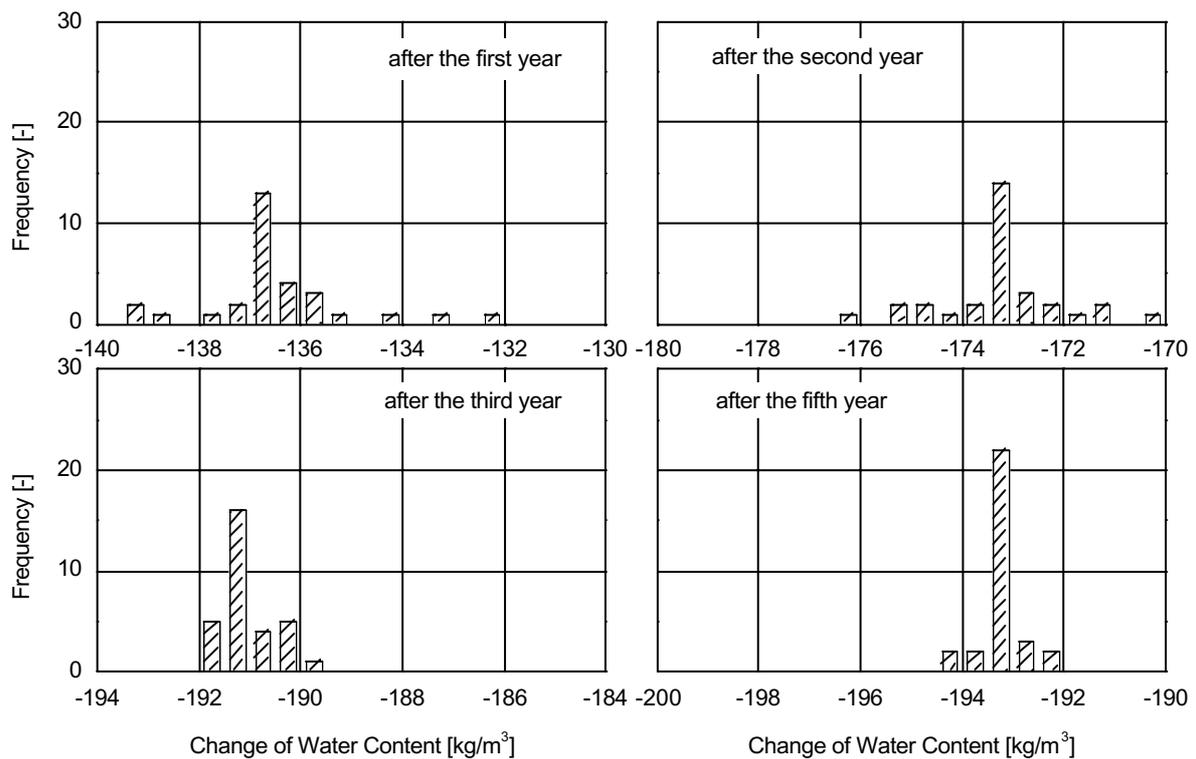
**Figure 4:** Frequency distribution of the change of water content since beginning after the first, second, third and fifth year. (Interval width:  $0.1 \text{ kg/m}^3$ )
