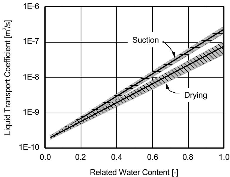
**Figure 2:** With uncertainty of the material parameters as shown in table 1 the hatched area represents the possible range of the approximated liquid transport coefficients for suction and drying.
