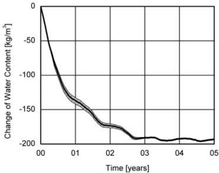
**Figure 3:** Material sensitivity analysis for the transient drying behaviour of the AAC flat roof under typical climate conditions for Holzkirchen. Each material parameter was changed from  $P$  to  $P + \Delta P$  respectively from  $P$  to  $P - \Delta P$ , giving a total of 25 simulations.
