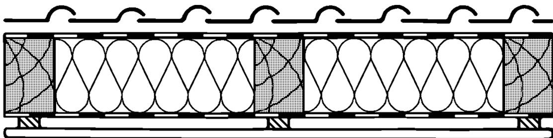
Figure 2 Typical construction of an unvented cathedral ceiling with fibre insulation between breather membrane (top) and vapour retarder (bottom).
