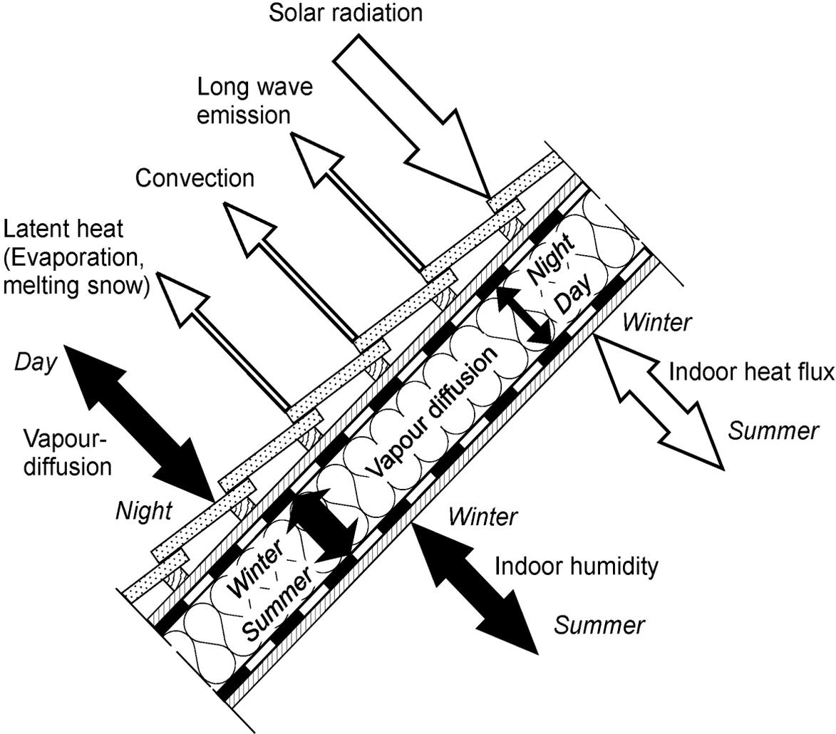
Figure 1 Transient hygrothermal loads and fluxes in and around an insulated roof assembly.
