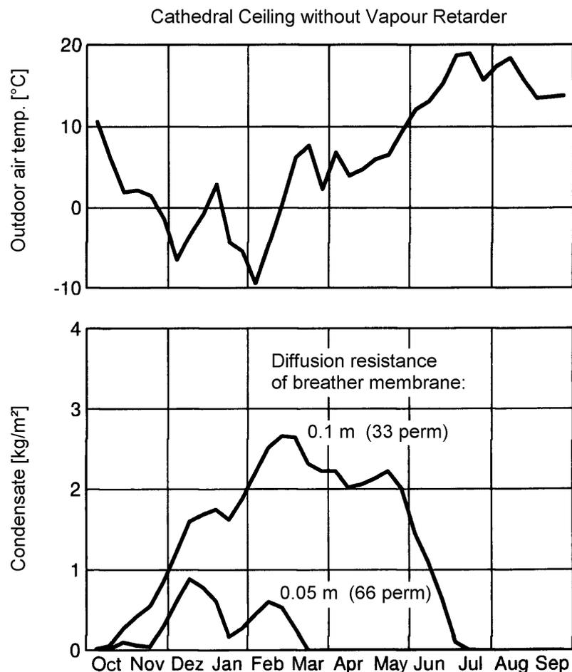
Figure 3 Measured outdoor temperature and calculated amount of condensate in the roof assembly without vapour retarder based on WUFI-simulations without solar radiation effects (worst case).
