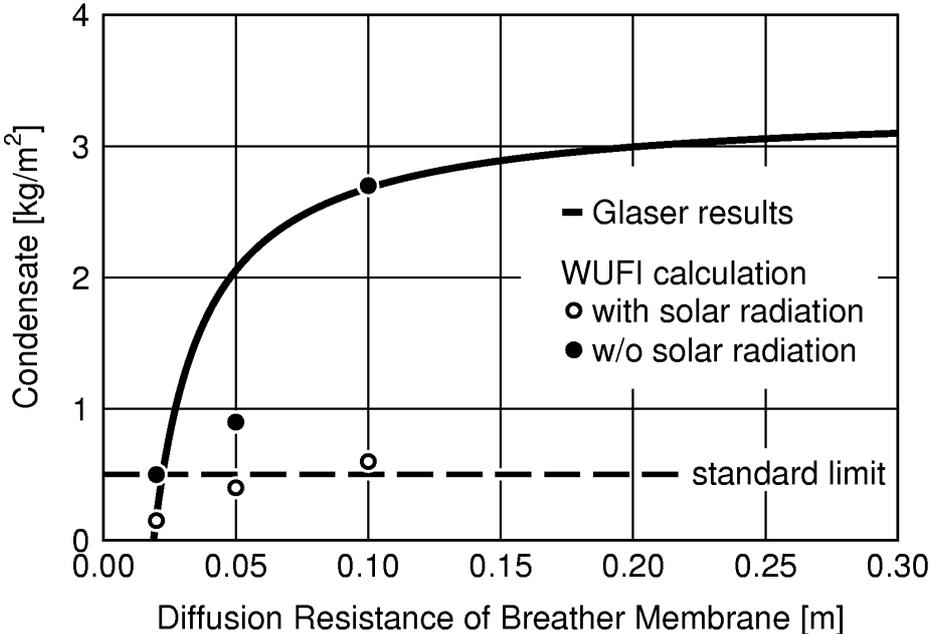
Figure 4 Interstitial condensate formed during the heating period in a cathedral ceiling without vapour retarder depending on the diffusion resistance of the breather membrane. The Glaser result (solid line) correspond to the simulation results taking the maximum amount of condensate from Figure 3 without solar radiation. If solar radiation for a south oriented roof without snow cover is considered, the condensation amount is reduced by drying intervals.
