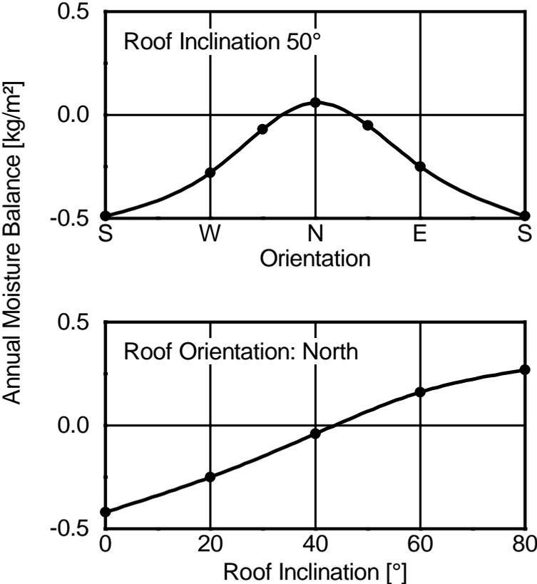
Figure 5 Annual moisture balance in a cathedral ceiling with vapour tight top and a slightly permeable vapour retarder ( $\mu d = 2 \text{ m}$ , 1.6 perm) determined with WUFI for different orientation and inclination of the roof.
