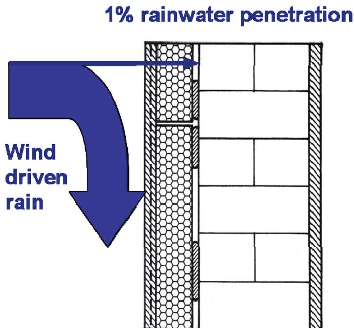
FIG 1. Example that shows the most likely deposit location for rainwater penetrating through leaks at joints and connections of a masonry wall with ETICS
