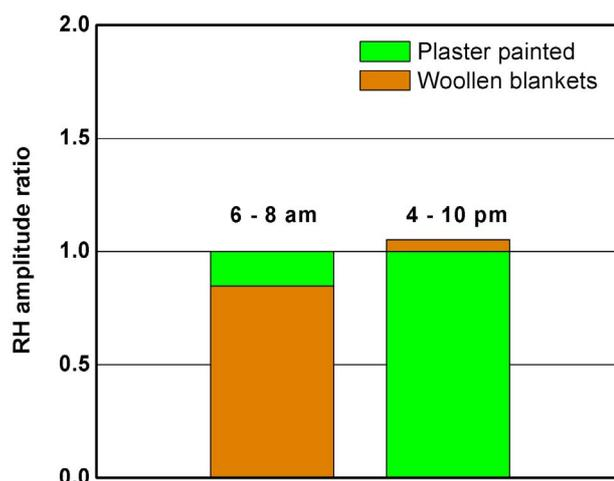
Fig. 55: Mean indoor air humidity amplitudes in the unlined test room with suspended woollen blankets, related to the conditions in the plastered reference room during the moisture production peaks in the morning (left hand) and evening hours (right hand).
