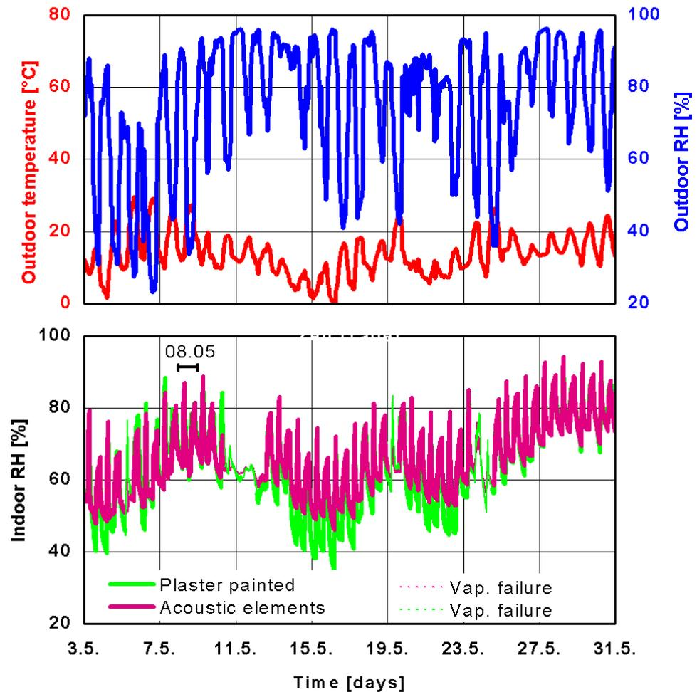
Fig. 33: Patterns of the recorded exterior climatic conditions and of the relative humidity in the test rooms during the measurement period.
