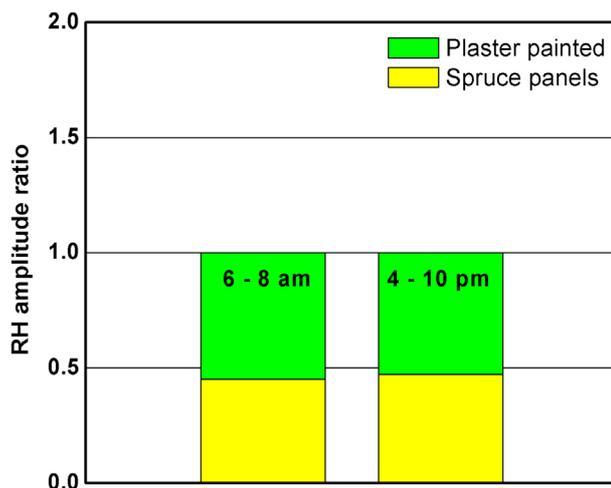
Fig. 29: Mean indoor air humidity amplitudes in the test room with spruce panels, related to the conditions in the reference room during the moisture production peaks in the morning (left hand) and in the evening (right hand).
