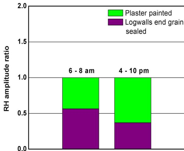
Fig. 45: Mean indoor-air humidity amplitudes in the test room supplied with the round-log units (ends sealed), related to the conditions in the reference room during the moisture production peaks in the morning (left hand) and in the evening hours (right hand).
