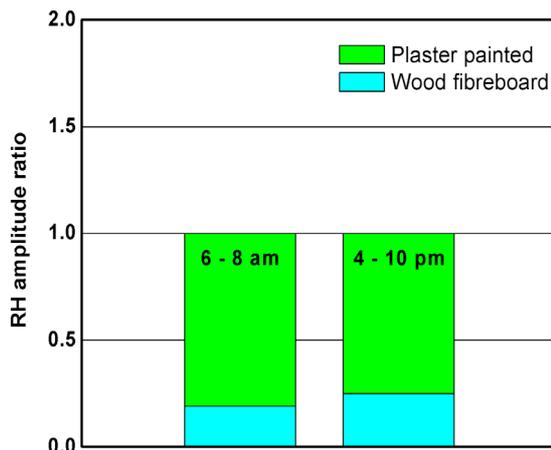
Fig. 50: Mean indoor air humidity amplitudes in the test room covered with fibreboard lining, related to the conditions in the reference room during the moisture production peaks in the morning (left hand) and in the evening (right hand).
