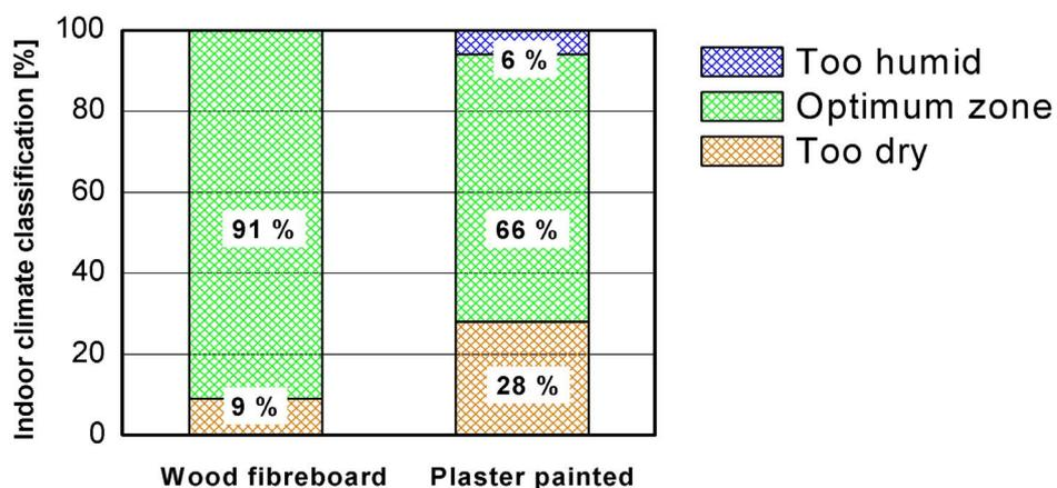
Fig. 51: Classification of the humidity conditions in the test room lined with fibreboard sheets and in the reference room (plastered) according to Fig. 1.
