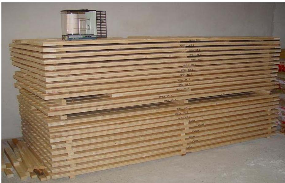
Fig. 12: Storage of spruce panels during the preconditioning phase.
