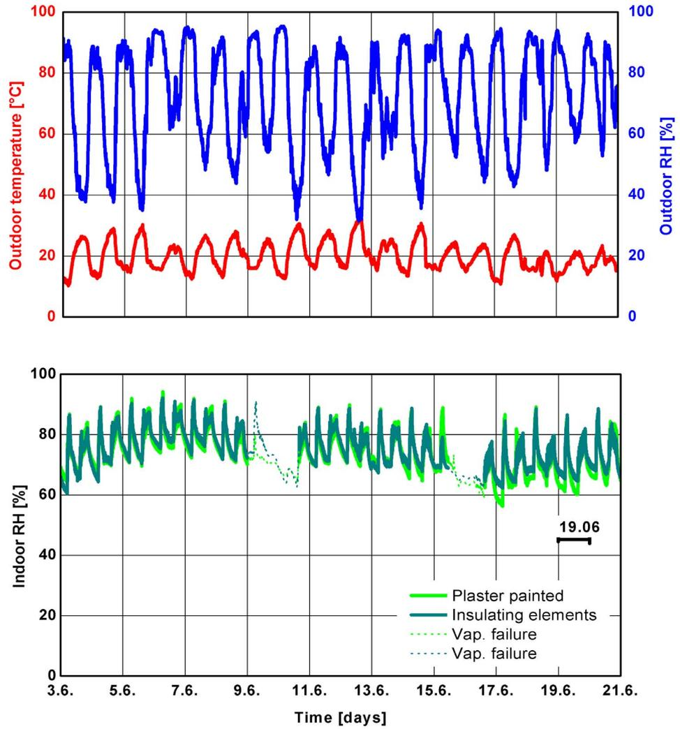
Fig. 37: Curves of exterior climatic conditions and relative humidity in the test room containing insulating units and in the reference room during the measurement cycle.
