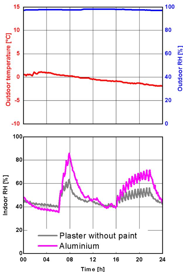
Fig. 14: Measured time profiles of the indoor air humidity in the non-hygroscopic test room and in the reference room (unpainted interior wall plaster).
