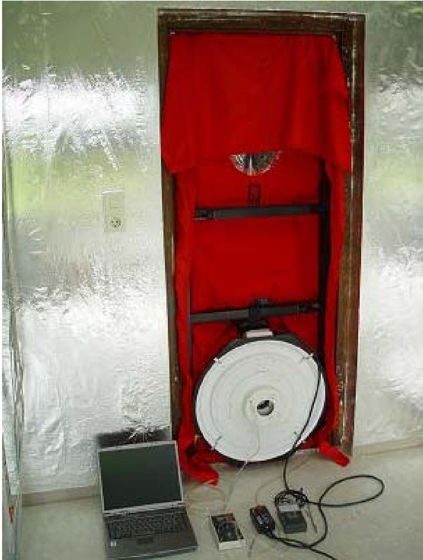
Fig. 6: Blower-door measurements.
