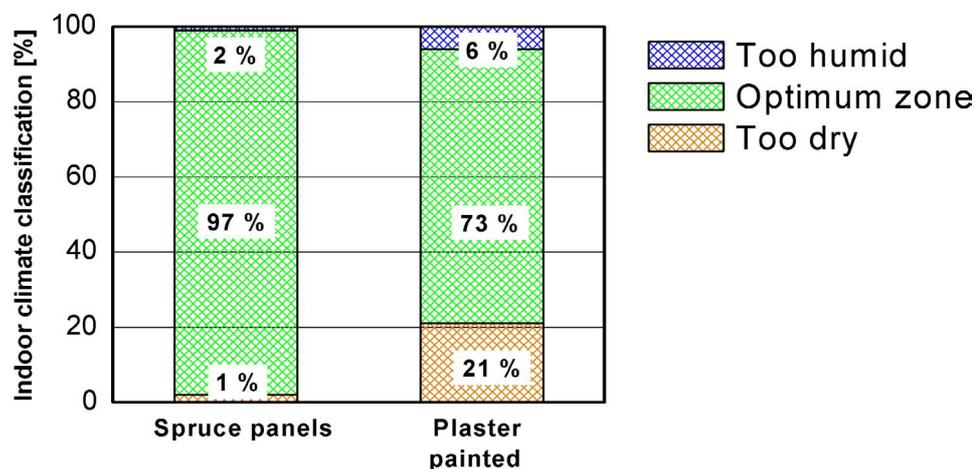
Fig. 30: Classification of moisture conditions in the test room lined with spruce panels and in the reference room (plastered) according to Fig. 1.
