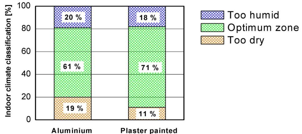
Fig. 23: Classification of the humidity conditions prevailing in the test room (aluminium foils) and in the reference room (plastered) after remaining in the optimum humidity range (30 - 55 % RH), respectively above it (too humid) and below it (too dry), according to Fig. 1.
