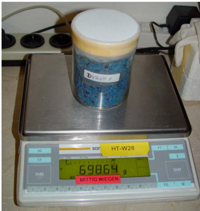
Fig. 13: Weighing a plaster sample to determine the  $s_p$ -value of the paint
