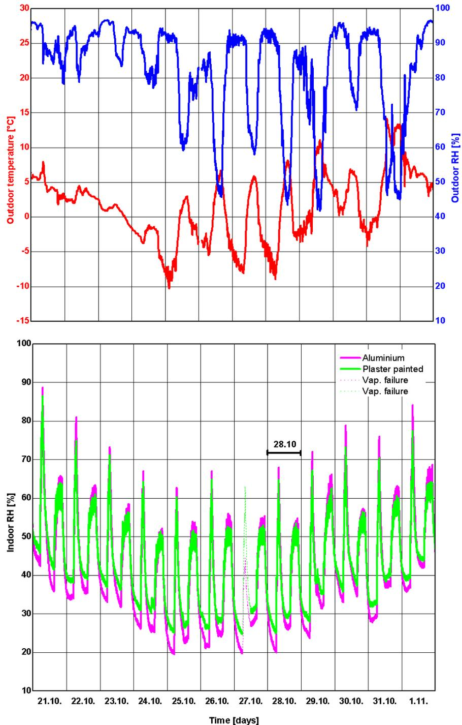
Fig. 17: Patterns of the exterior climatic boundary conditions (top) and the indoor air humidity in the test rooms (bottom).
