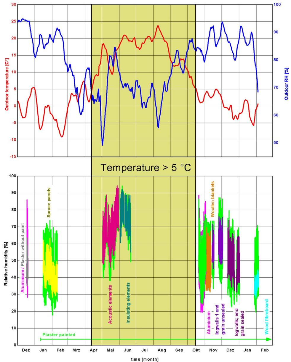
Fig. 24: Overall survey of the test period. The recorded exterior climatic boundary conditions are presented as floating decade mean.
