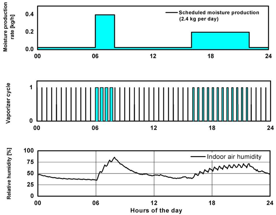
Fig. 8: Diurnal moisture production pattern in the experimental rooms
