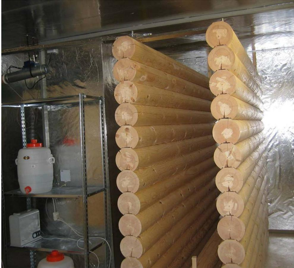
Fig. 40: Photograph of the round-log walls mounted in the test room.
