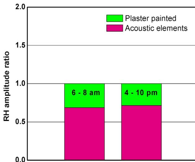
Fig. 35: Mean indoor air humidity amplitudes in the test room containing acoustic elements, related to the conditions in the reference room during the moisture-production peaks in the morning (left hand) and in the evening (right hand).
