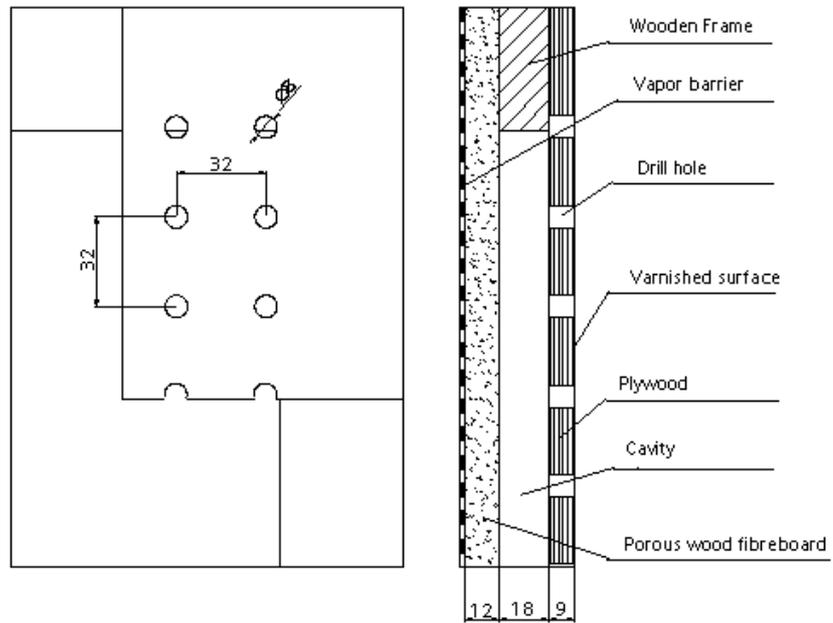
Fig. 32: Detailed drawing of an acoustic element.
