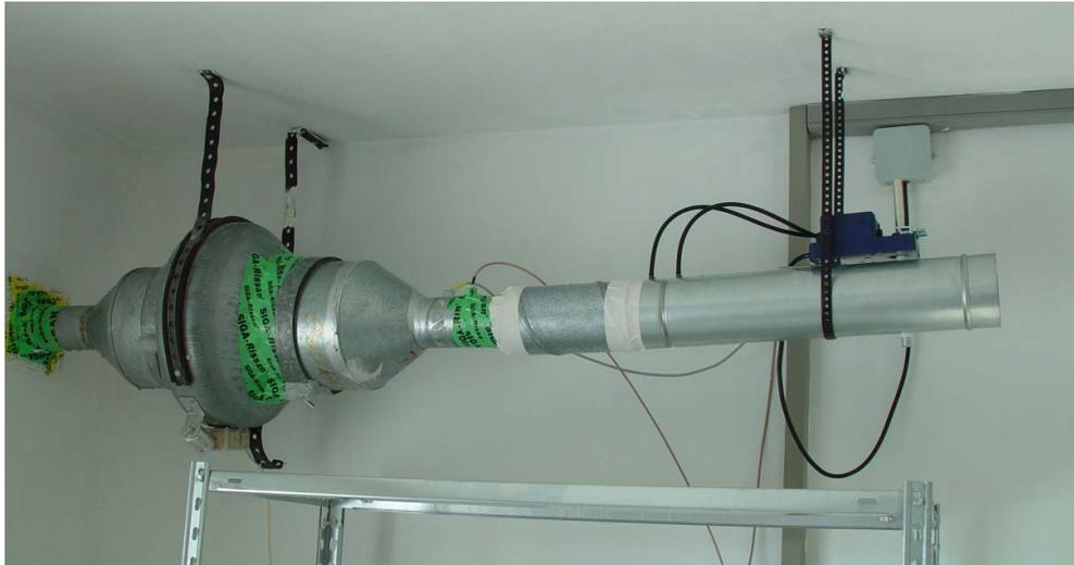
Fig. 7: Blowers for maintaining continuous ventilation rate of 25 m<sup>3</sup>/h.
