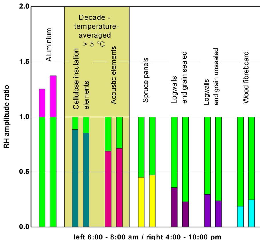
Fig. 52: Compilation of the determined mean humidity amplitude in the test room, related to the situation in the reference room and considering the respective projected surface area of the test room linings.
