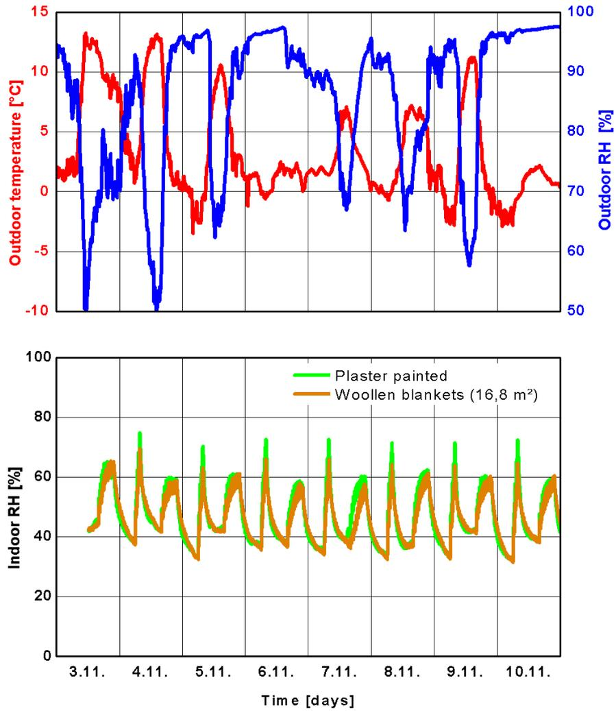
Fig. 53: Time-profiles of exterior climatic conditions and relative humidity in the unlined test room containing woollen blankets and in the plastered reference room during the 8-day measurement period.
