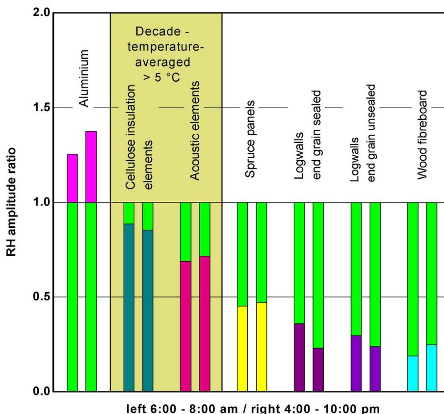
Fig. 52: Compilation of the determined mean humidity amplitude in the test room, related to the situation in the reference room and considering the respective projected surface area of the test room linings.
