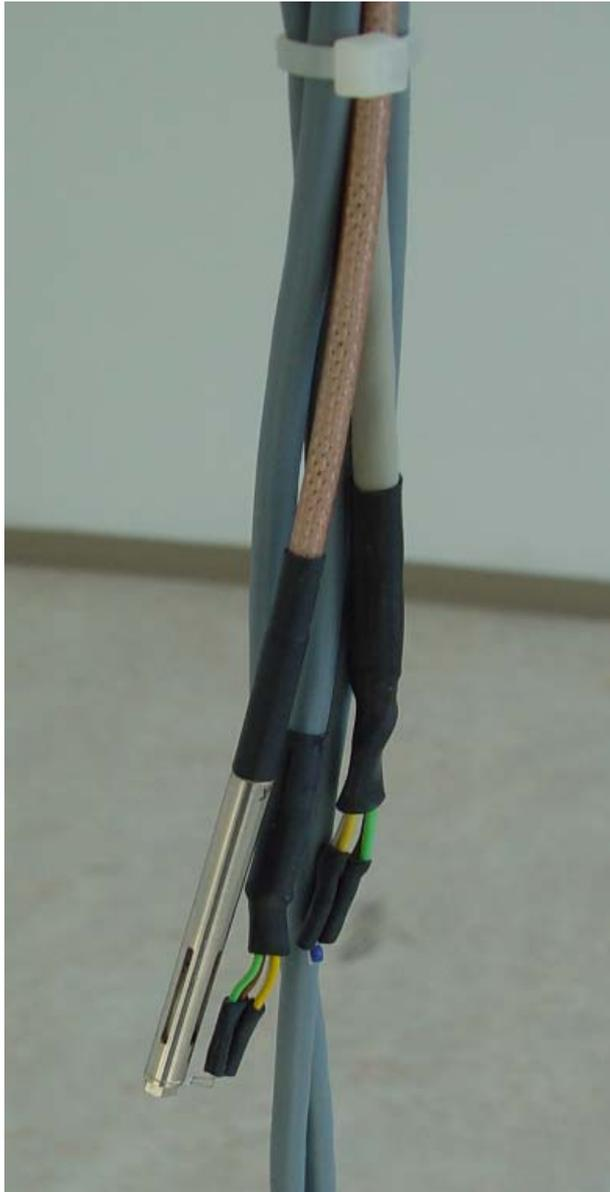
Fig. 10: Humidity and temperature sensors in the centre of the room.
