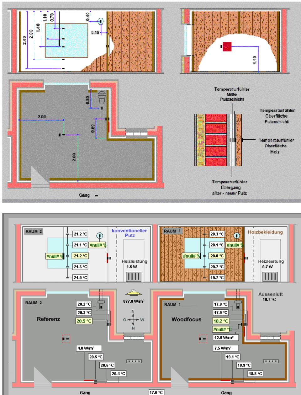
Fig. 11: Visualisation of the experimental rooms; location of sensors and representation of measured data.
