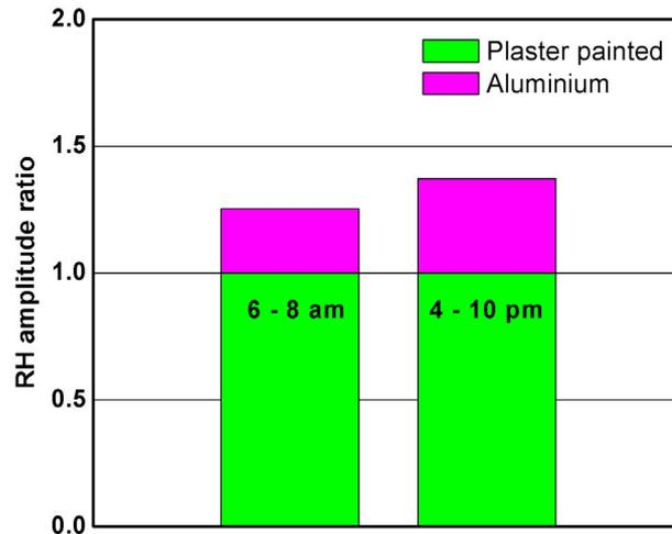
Fig. 22: Average of the related humidity peaks from Fig. 21 during the 12-day test period.
