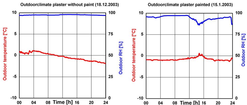
Fig. 16: Measured curves of the outside air conditions on winter days that were selected to compare the moisture buffering effects of the interior plaster in the reference room before and after painting.
