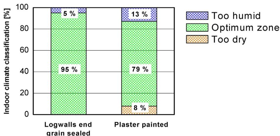
Fig. 46: Classification of the moisture conditions in the test room supplied with round-log wall units (ends sealed) and in the reference room (plastered) according to Fig. 1.
