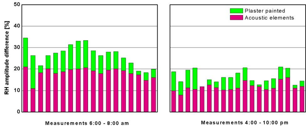
Fig. 34: Indoor air humidity amplitudes in the test rooms containing acoustic elements resp. interior plaster during the moisture-production peaks in the morning (left hand) and in the evening (right hand).
