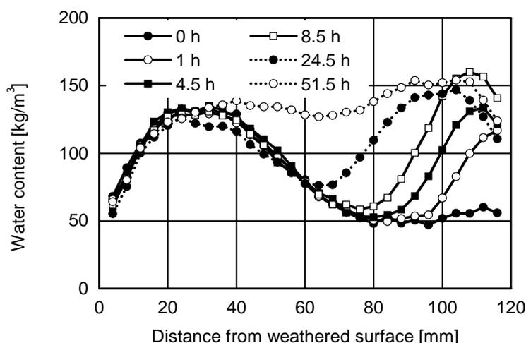
Fig. 10: Moisture profiles of the concrete specimen after the water absorption test in Fig. 9 by bringing the opposite side into contact with water.
