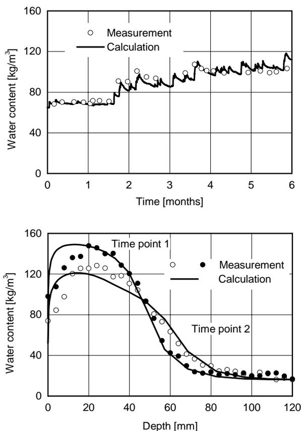
Fig. 6: Measured and calculated water contents of a prismatic concrete specimen exposed at the left hand side to natural weather during the first six months of the observation period. Top: Total water content determined by weighing and calculation. Bottom: Measured (NMR-scanning) and calculated moisture profiles.
