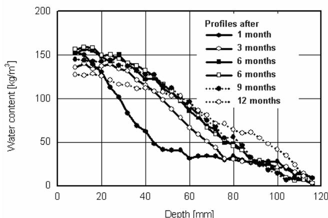
Fig. 8: Moisture profiles measured with the help of NMR at various times during the entire exposure period of the concrete specimen.
