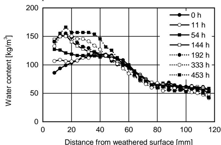
Fig. 9: Moisture profiles of the concrete specimen after the two-year weathering period determined by NMR-scanning during a laboratory water absorption test (formerly exposed side in contact with water).
