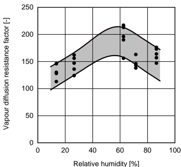
Fig. 3: Diffusion resistance factor of the different concrete specimens (reason for scatter see Fig. 2) plotted over mean ambient relative humidity (mean between the RH on both sides of the specimen).
