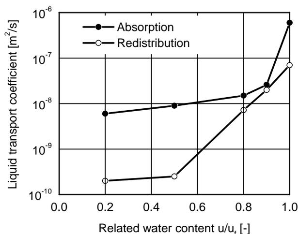
Fig.4: Transport coefficients for water absorption and redistribution determined from transient moisture content profiles. The water content at the x-axis is related to capillary saturation.
