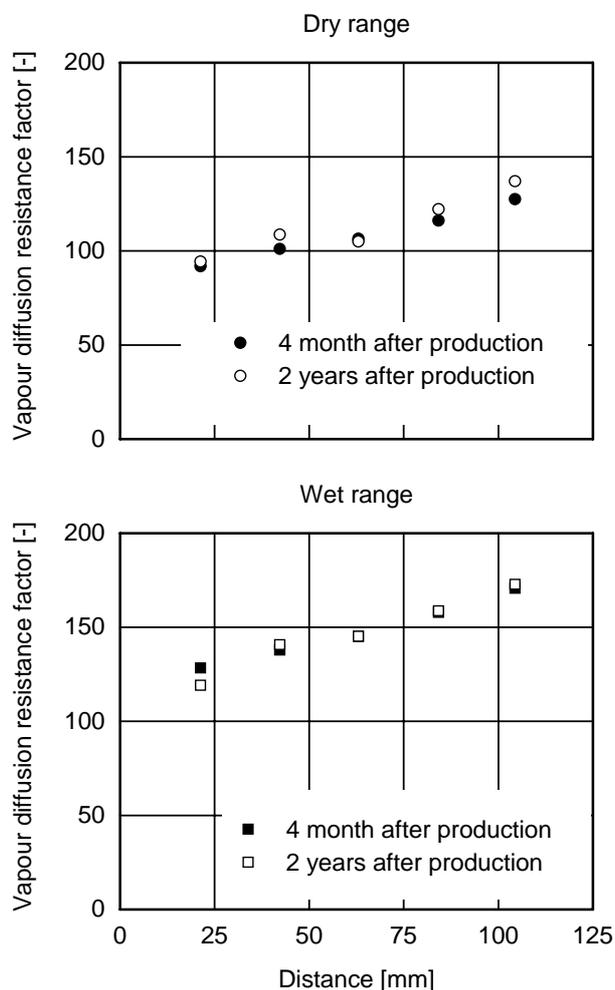
Fig. 2: Results of the dry-cup (top) and wet-cup (bottom) tests of 20 mm thick concrete slices taken from different positions in the original moulded cubes ( $x$ -axis indicates the original distance of the specimens from the cube's upper surface before it had been cut to prepare the specimens). The tests were repeated 2 years later to check the effect of carbonation.
