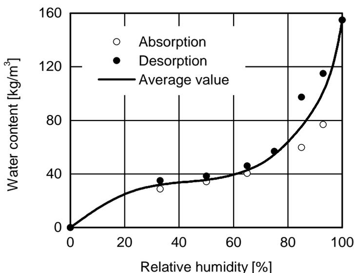
Fig. 1: Results of ab- and desorption tests performed on the investigated concrete samples including the average sorption isotherm which will serve as input for the simulations.
