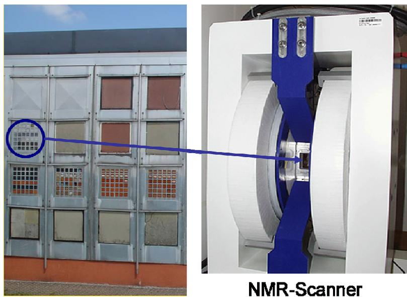
*Fig. 5: Photographs of the concrete specimens exposed at the west oriented façade of a 4 m high test hall (left) and of the NMR-scanner which was used to determine the moisture profiles of the exposed specimens at certain points in time.*
