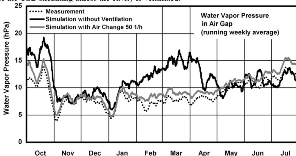
Fig. 1. Vapour pressure variations in the 19 mm thick air gap beneath the stucco calculated with and without ventilation in comparison to measured data from the ventilated cavity wall of the WSU test building [12].
