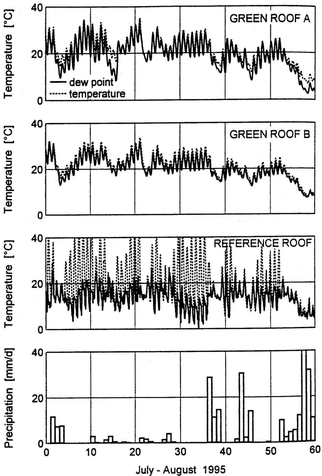
Fig. 4 Temperatures and dew point temperatures measured above the insulation layer in the test roofs as well as daily precipitation values in the period of July and August 1995.
