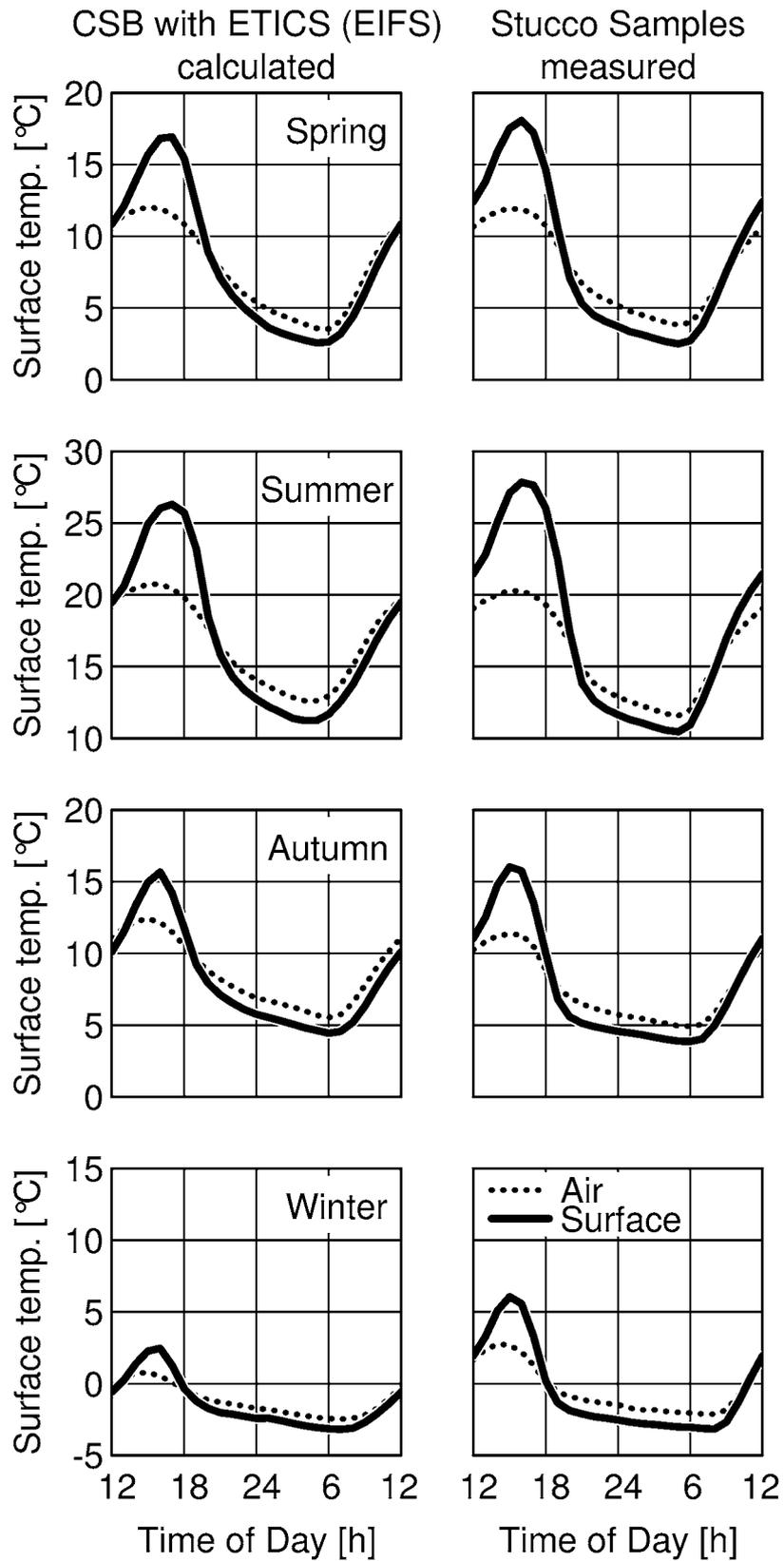
Fig. 1: Average diurnal surface temperature cycles for an ETICS.
