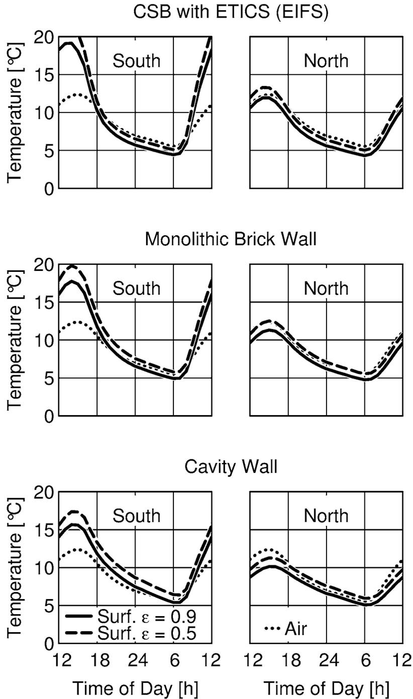
Fig. 2: Calculated average diurnal surface temperature cycles for different wall constructions.
