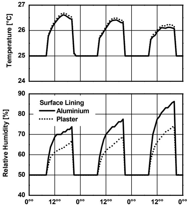
Figure 9: Simulated indoor temperature and relative humidity during the observation period in March (Bangkok climate).
