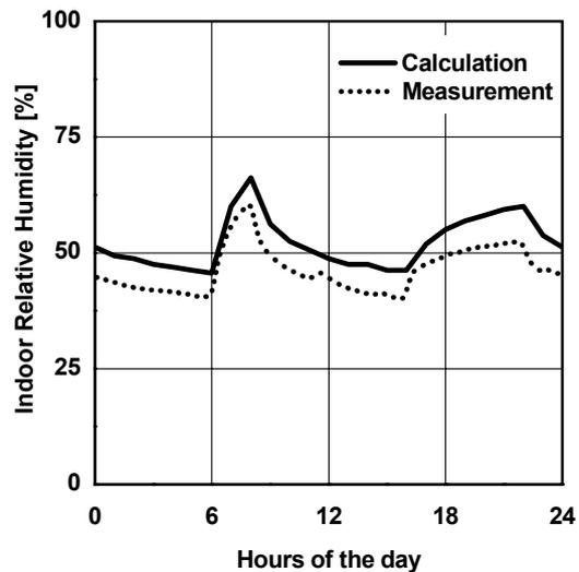
Figure 6: Simulated and measured evolution of the indoor air humidity during a diurnal cycle in the reference room coated with a lime-gypsum interior plaster.
