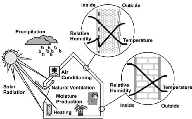
Figure 1: Coupling concept for the simultaneous treatment of the hygrothermal effects of interior heat and moisture loads, exterior climate and transient behaviour of envelope components.
