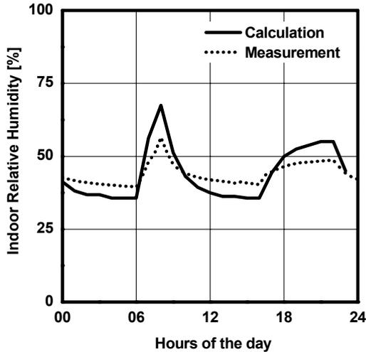
Figure 7: Simulated and measured evolution of the indoor air humidity during a diurnal cycle in the test room when walls and ceiling were covered with wooden panels.
