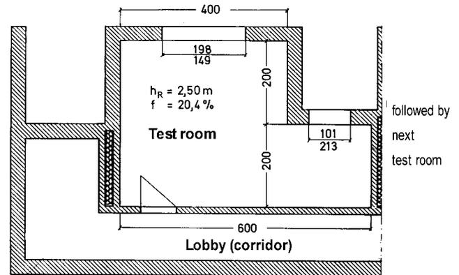
Figure 2: Ground plan of the test room.
