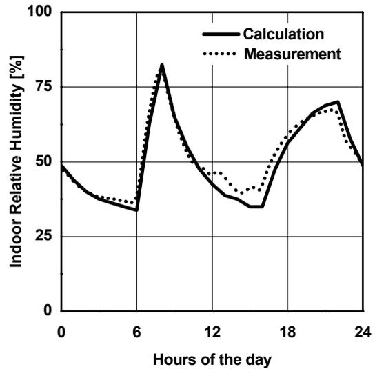
Figure 5: Simulated and measured evolution of the indoor air humidity during a diurnal cycle in the test room coated with aluminium foil.
