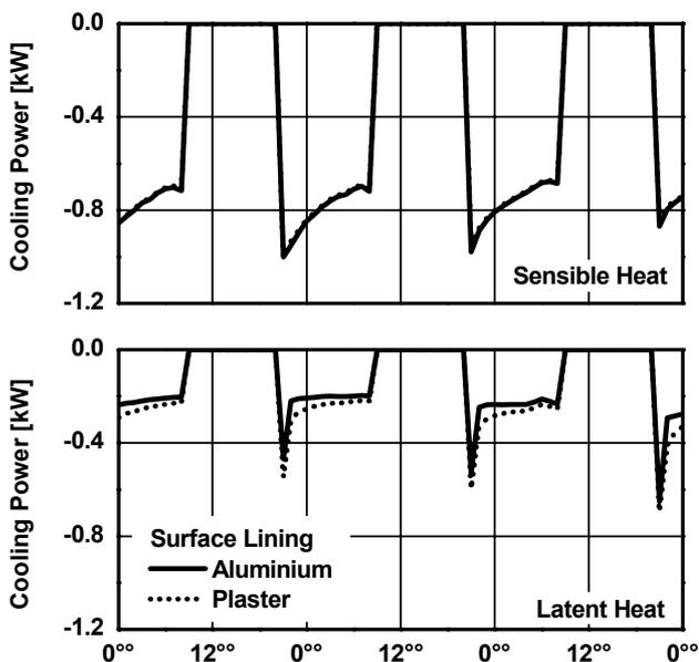
Figure 10: Sensible and latent cooling load to be removed in the different rooms by the AC-system during the observation period.
