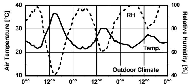
Figure 8: Outdoor air temperature and relative humidity recorded for Bangkok in March (3 day observation period).
