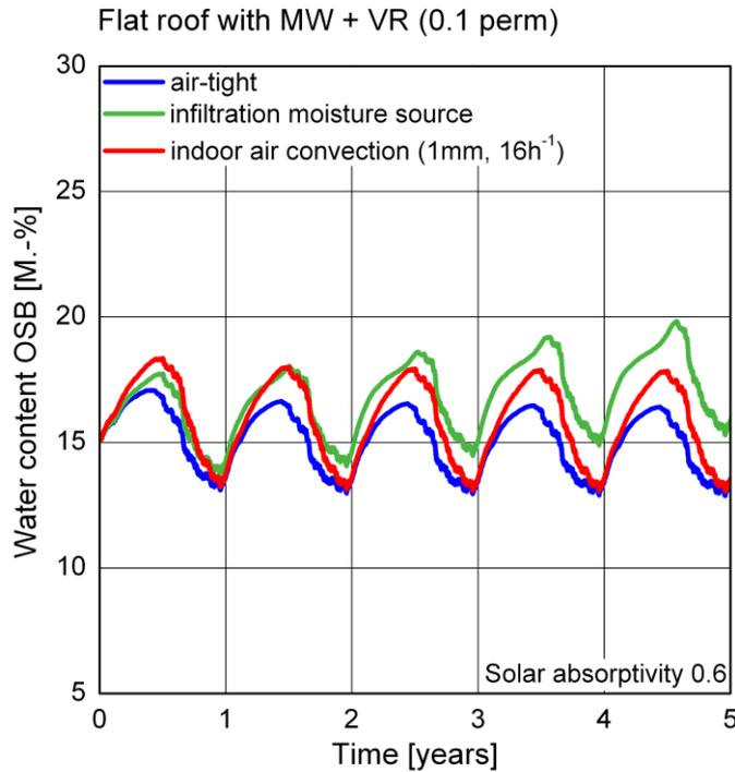
FIGURE 4: Calculation results as in Figure 3 with the difference that the permeance of the vapour retarder has been increased by a factor of 10.
