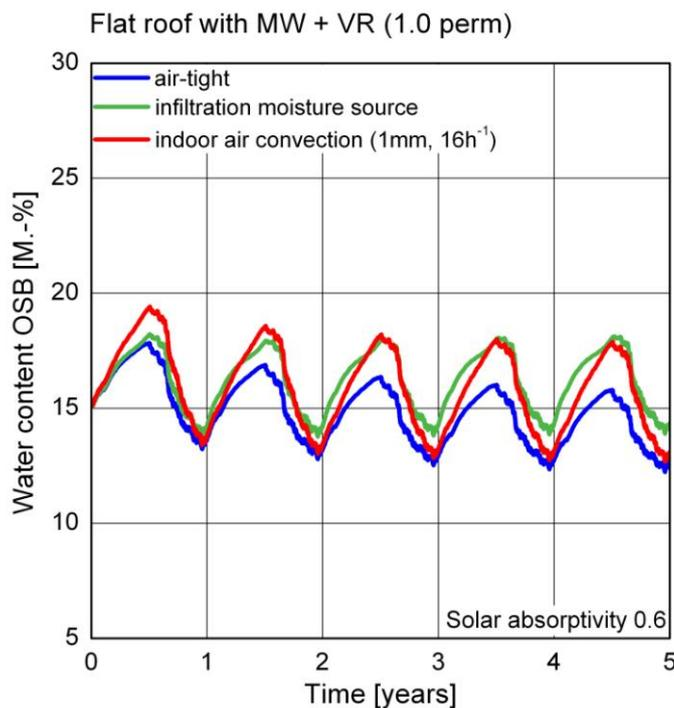
FIGURE 6: Calculation results as in Figure 5 with the difference that the permeance of the vapour retarder has been decreased by a factor of 10.
