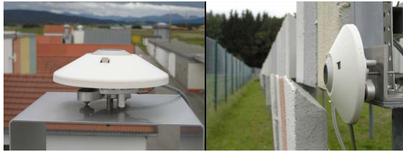
FIG. 3: Horizontal (left) and vertical (right) pyrometers at the IBP test site.
