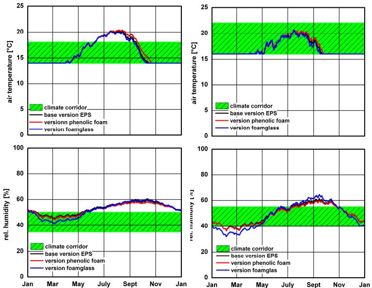
Figure 3: Comparison of the hygrothermal behavior of the three constructional versions, left for the archive depot and right for the depot of paintings.
