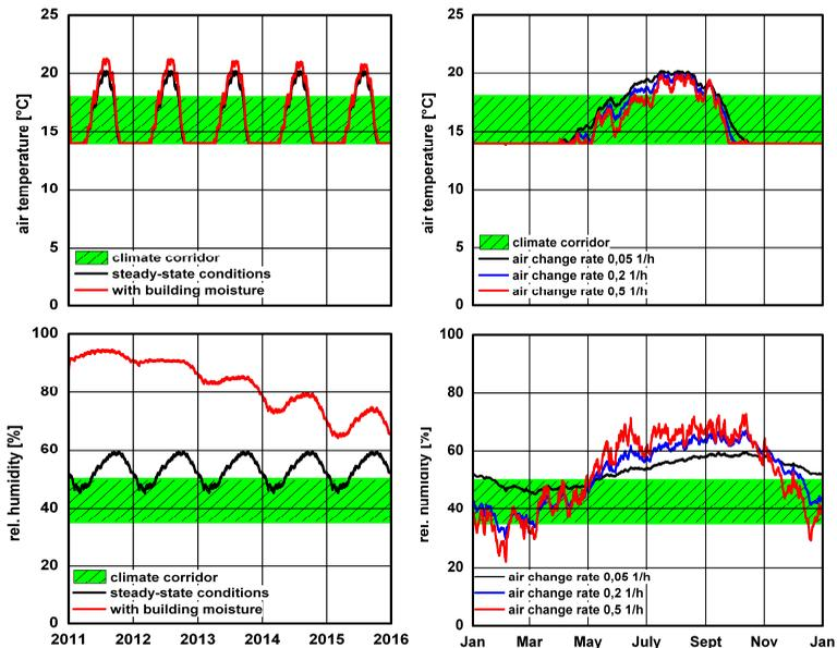
Figure 4 Hygrothermal impact of built-in moisture (left) and of the air change rate (right)
