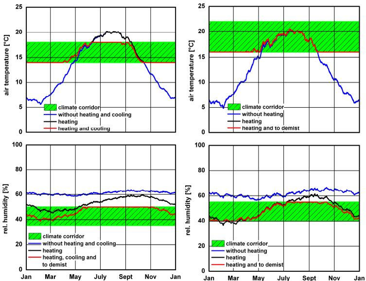
Figure 2 Hygrothermal behavior of basic version for variation of air-conditioning, left for the archive depot and right for the depot of paintings.
