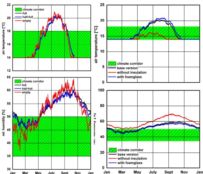
Figure 5: Hygrothermal impact of the archive material (left) and of the floor slab (right)
