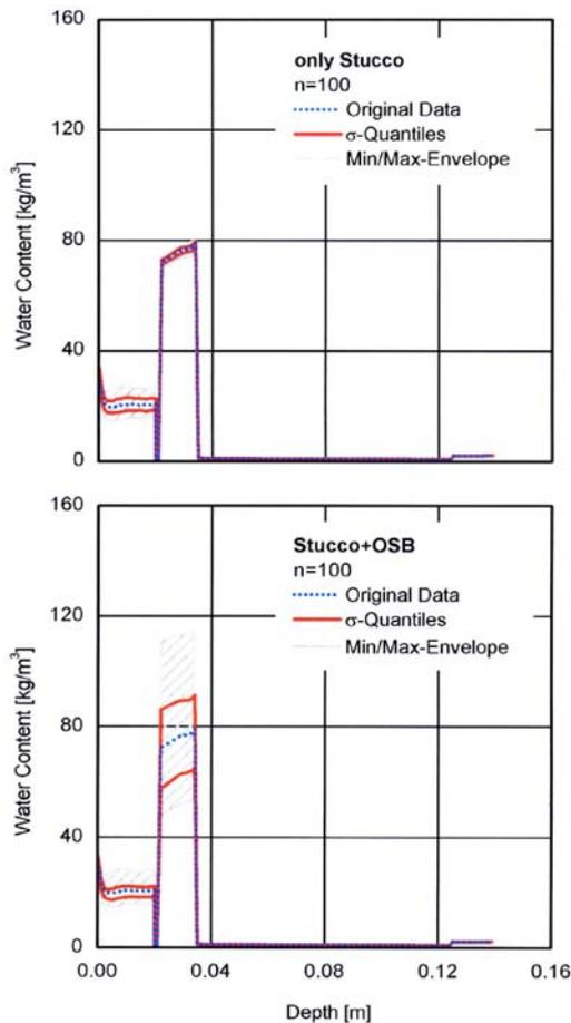
**Figure 1** Water content profiles at the end of the simulation. Deterministic solution (dotted line), the minimum and maximum values with  $\sigma$ -quantiles. Top figure: only the properties of stucco were varied. Bottom figure: the properties of both stucco and OSB were varied.
