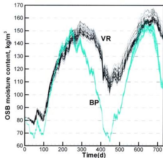
**Figure 4** Moisture content of the OSB layer as a function of time for “series 2” simulations. Starting date July 1. BP: cases with building paper under gypsum board; VR: cases with 6-mil polyethylene under gypsum board. Two years of simulation, with first year = coldest and second year = warmest.
