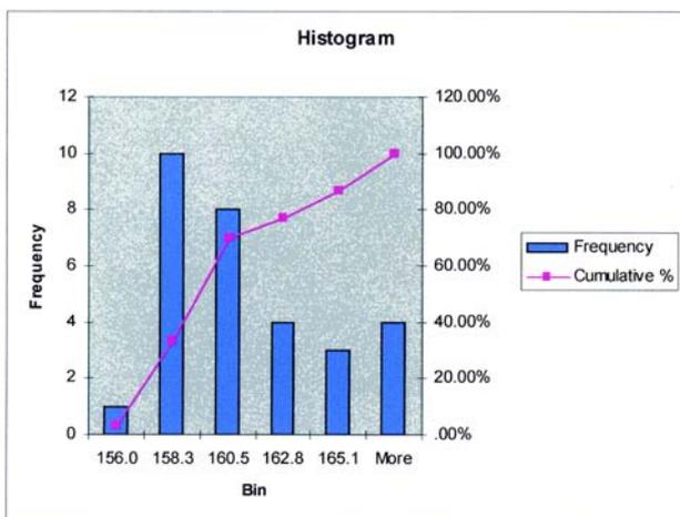
**Figure 5** Histograms of moisture content of OSB in 30 stochastic runs. Moisture content in the OSB at the beginning of May after nearly two years (667 days) of simulations when the moisture contents are highest. Top: cases with building paper. Bottom: cases with vapor retarder. Average moisture contents of 30 runs: with building paper, 152.8 kg/m<sup>3</sup>; with vapor retarder, 160 kg/m<sup>3</sup>.
