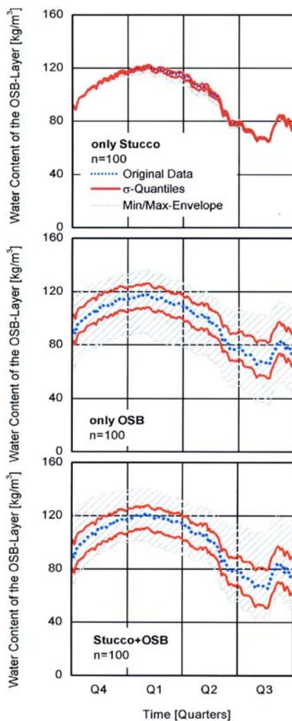
**Figure 3** Water content of the OSB layer as a function of time. Deterministic solution (dotted line), the minimum and maximum values with  $\sigma$ -quantiles. Top figure: only the properties of stucco were varied. Middle figure: only the properties of OSB were varied. Bottom figure: the properties of both stucco and OSB were varied.
