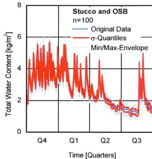
**Figure 2** Total water content as a function of time. Deterministic solution (dotted line), the minimum and maximum values with  $\sigma$ -quantiles. The properties of both stucco and OSB were varied to produce these results.
