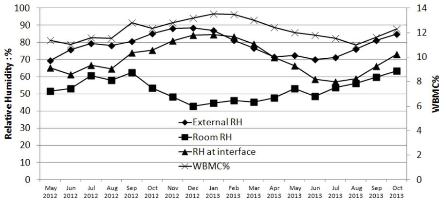
FIG 6. Relative humidities measured externally, within the flat and at interface stonework / insulation (average of 5 measurements); WBMCs measured at the same interface (average of 5 measurements)
