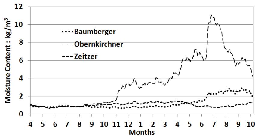
FIG 9. Overall moisture content of the mineral wool insulation
