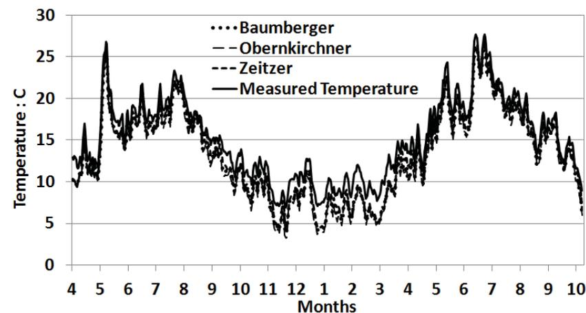
FIG 10. Temperature in the outer 1 mm of the mineral wool insulation (i.e. near interface of stonework and insulation) with the measured data
