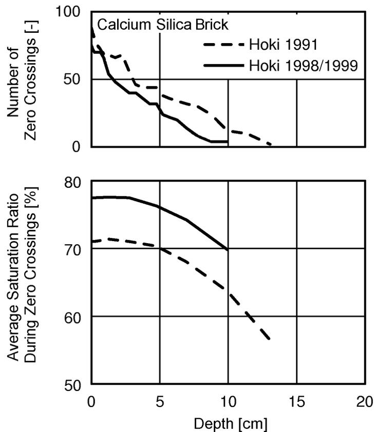
**FIGURE 3:** Number of zero crossings in calcium silica brick with defect paint coating as distributed over the building element's cross-section (top) and the resulting average saturation ratio (bottom).
