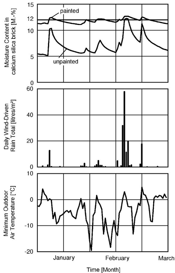
**FIGURE 2:** Course in time for the moisture content of the 5 cm thick outer surface zone of a calcium silica brick wall with defect paint coating as well as on a non-coated example, with specifications of the daily total of wind-driven rain and the minimum daily outdoor air temperature.
