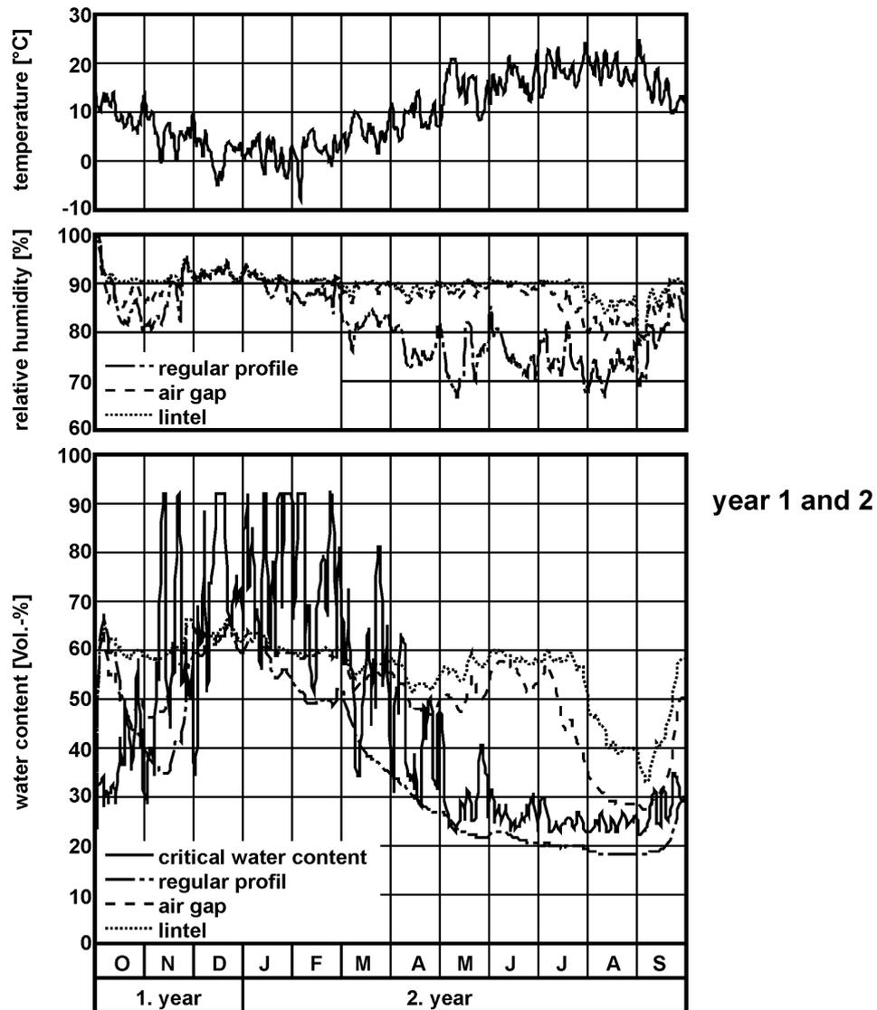
Figure 1: Courses of the temperature (top) and the relative humidity (middle) as well as the water content of the spores (bottom) at different façade positions on the exterior stucco, calculated for a wall of concrete insulated with ETICS.
