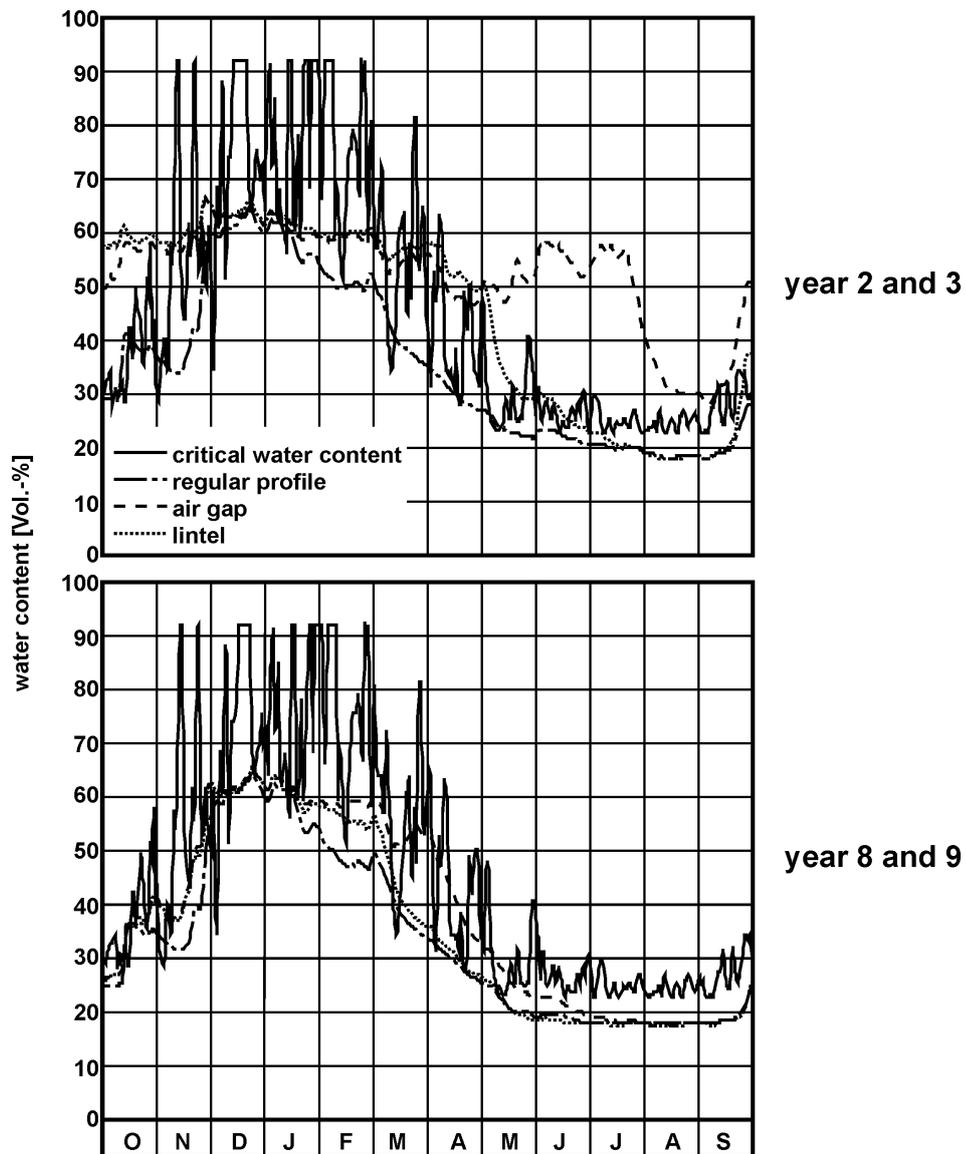
Figure 2: Courses of the water content of the spores at different places on the exterior stucco of an exterior wall in the second (top) and in the eighth year of examination (bottom), calculated for a wall of concrete insulated with ETICS.
