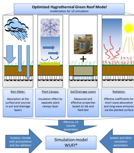
Figure 2: Input and transfer parameters of the optimized hygrothermal green roof model
