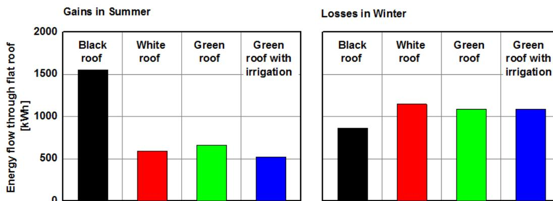
Figure 7: Energy gains and losses through the flat roof with black or white roofing membrane or greenery.
