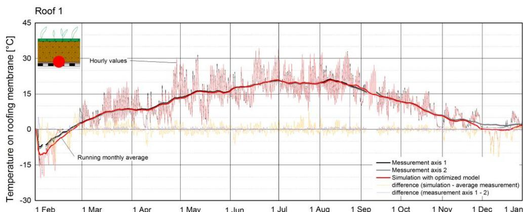
Figure 3: Comparison of the measured and simulated temperatures beneath green roof 1
