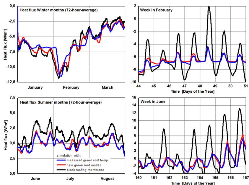
Figure 5: Heat fluxes through the roof in summer and winter simulated based on the measured temperatures beneath the green roof (blue) and the new green roof model (red) compared to the heat fluxes of a black membrane roof (black).
