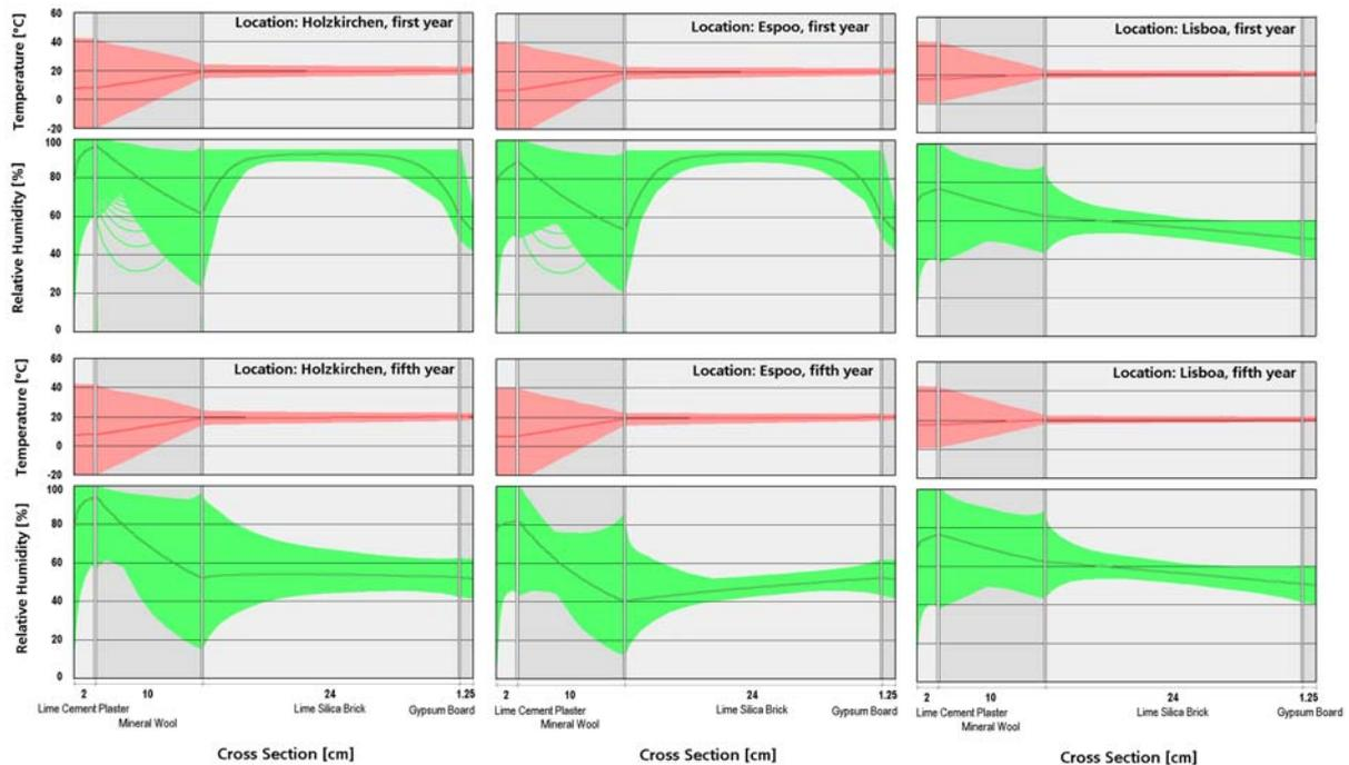
**Figure 2: West facing façade at the three different locations Holzkirchen (left), Espoo (middle) and Lisboa (right). Variation range and average profile of temperature (red) and relative humidity (green) in the facade during the first (top) and the fifth (bottom) year of the simulation.**
