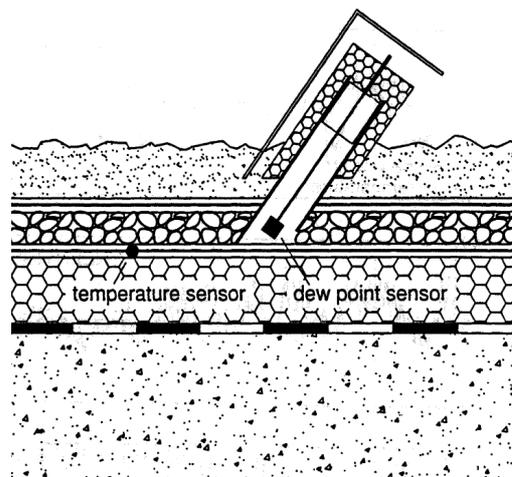
**Figure 1.** Schematic figure showing the positions of the temperature and dew point sensors in the drainage layer of the green roof.
