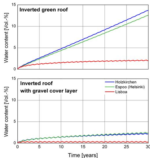
**Figures 5 (top) and 6 (bottom).** Simulated water content of the insulation boards in inverted roofs with vegetation (green roof Fig. 5) and gravel cover layer (Fig. 6) at Holzkirchen (Germany), Espoo (Helsinki, Finland) and Lisboa (Portugal) over a period of 30 years.
