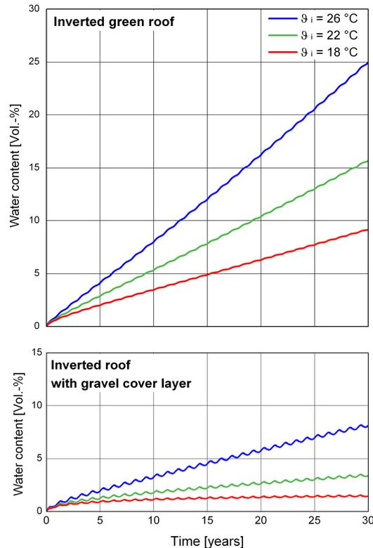
**Figures 7 (top) and 8 (bottom).** Simulated water content of the insulation boards in an inverted roof with vegetation (Fig. 7) and gravel cover layer (Fig. 8) at Holzkirchen with different indoor temperature levels of constant 18, 22 and 26 °C.
